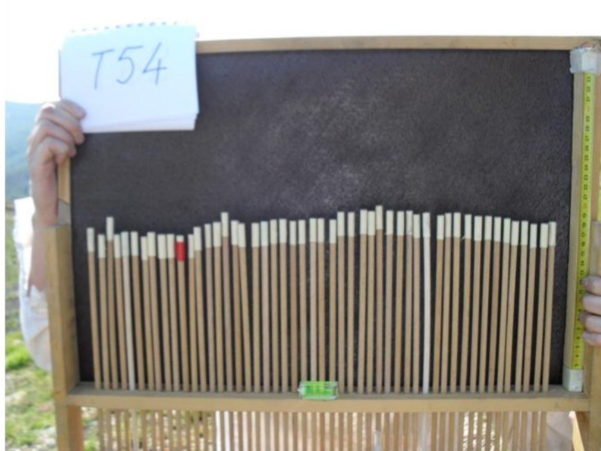
Figure 3.6 – Pinmeter, showing the readings of the roughness of the soil (tip of the pins)
