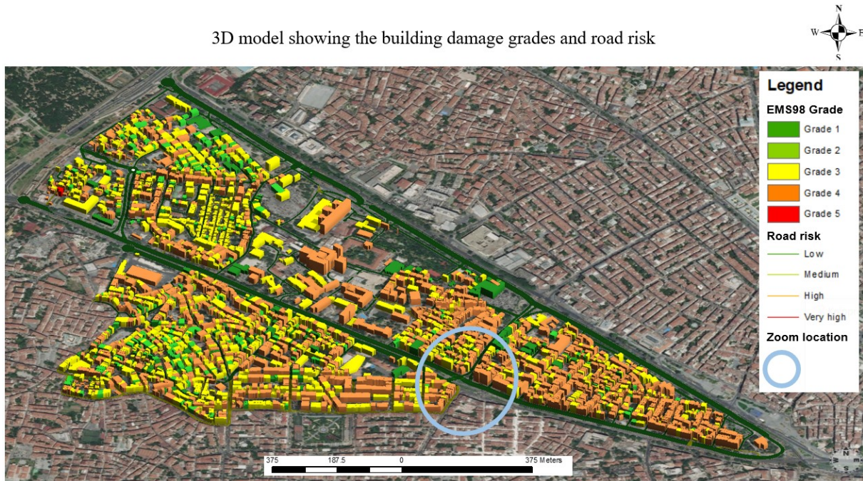
Figure 33: Picture of the 3D model scene showing the building damage grades and road risk for the entire case study area. The blue circle refers to the zoomed-in location in Figure 34. Link to the web scene: https://bit.ly/3KJiv7c . Source: Author (2022)
