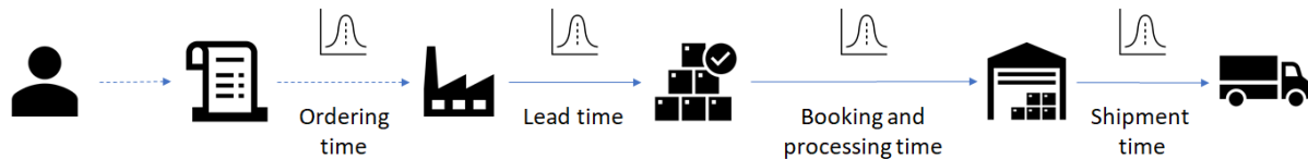
Figure 7: Visualisation of ordering and delivering process of a non-SKU
