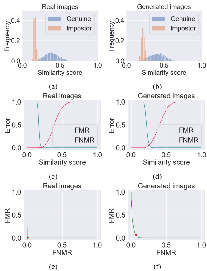
Fig. 15: Genuine and impostor similarity score distributions of the real dataset (a) and the generated image set (b). The respective plots of the FMR and FNMR over the classification error are given in (c) and (d). The corresponding DET-curves are given in (e) and (f).
