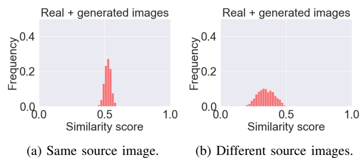
Fig. 16: Similarity scores between real and generated images. For (a), each generated image is compared with the corresponding original image. For (b), each generated image is compared with the real images of that same finger, skipping the ones corresponding to the exact same image (which are covered for (a)). The mean for (a) is 0.520 \pm 0.023 , and for (b) 0.352 \pm 0.065 .
