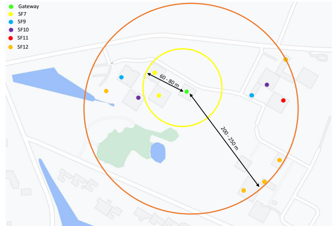
Fig. 7. Transmission range of different spreading factor numbers referenced as different colour points
