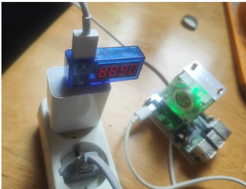
Figure 1: The setup used to measure the power consumption of the Raspberry Pi while running the different algorithms
