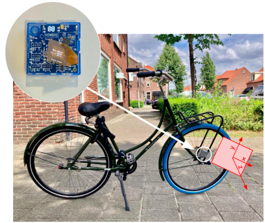
Fig. 3. Installation of the Nordic Thingy:52
