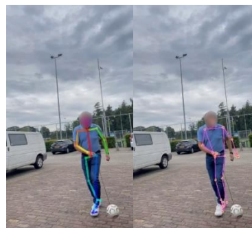
Figure 5: Example frames where BlazePose falsely detected lower body joints
