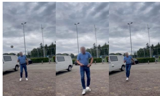
Figure 4: Example frames where YOLOv5 and EfficientDet struggled to detect the ball due to white background
