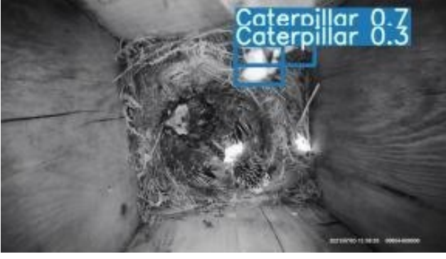
Fig. 11 Example of double detection fault.
