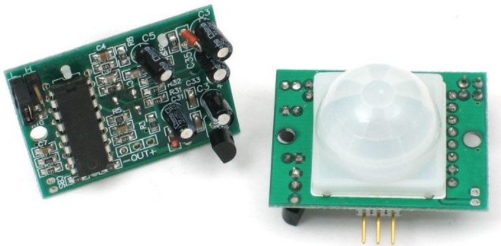
FIGURE 2: Passive Infrared Sensor for motion detection (PIR sensor) [21]
