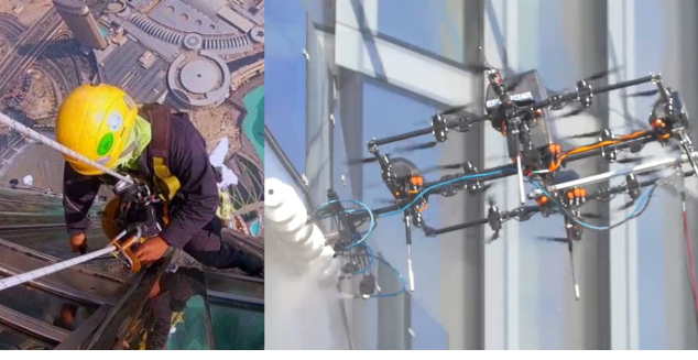
Fig. 1: A typical scenario where a worker is cleaning windows at a skyscraper (Left) URL as compared to an aerial robotic worker performs the same task (Right) URL .
