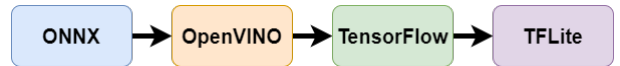
Figure 13: Conversion of ONNX model to TFLite model without addition of extra transpose layers.
