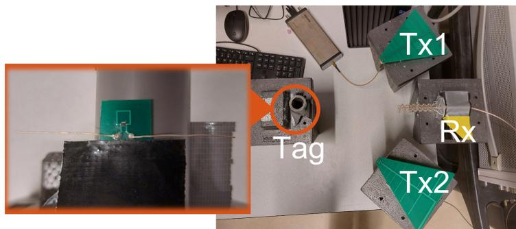
**Figure 4.2:** Picture of the measurement setup
