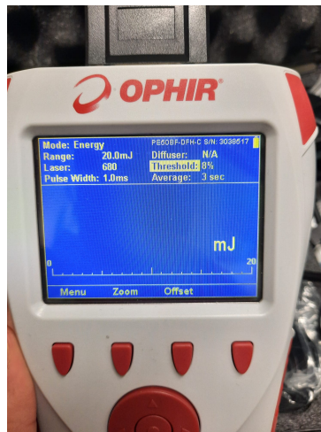
Figure 8: Settings for the power meter.
