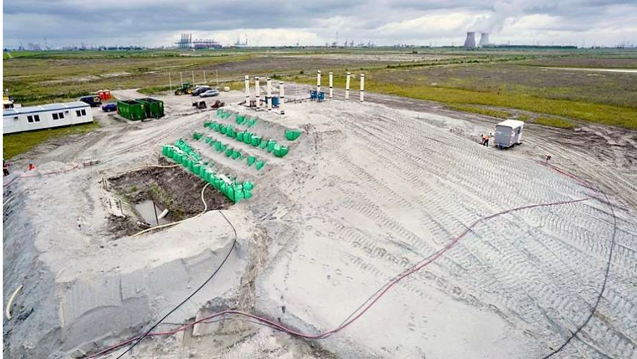
Figure 3.1: Experimental set-up at the LLHPP. The infiltration tubes can be seen on the top of the artificial dyke and the ditch of the North side of the dyke can be seen on the left side.
