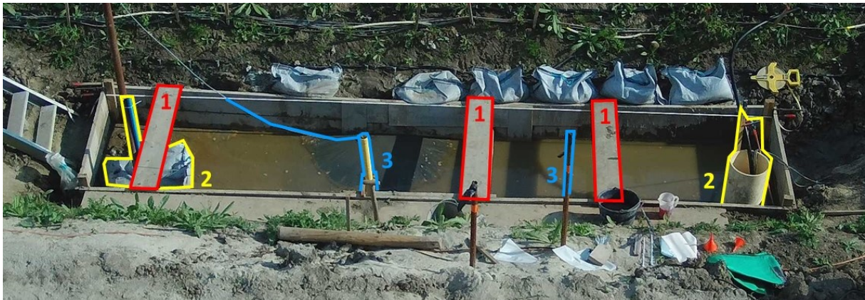
Figure 5.1: Obstacles inside of the ditch at the experimental set-up where the numbering corresponds to 1) wooden gangways 2) larger measurement devices and 3) small measurement devices.
