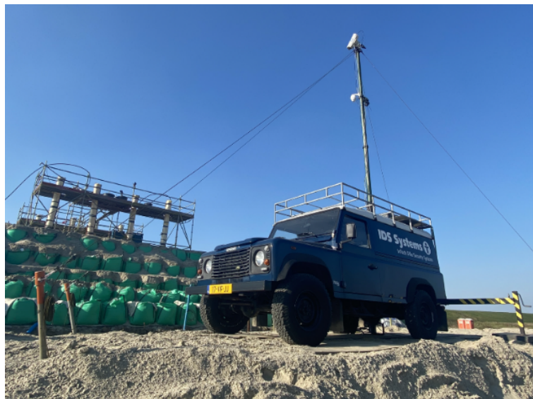
Figure 3.3: Set-up of the thermal imaging measurement device (Steenblik, 2021).
