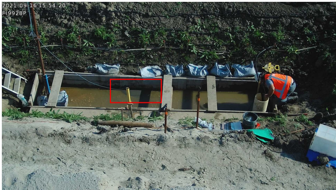
Figure A.3: A thermal (top) and RGB (bottom) image taken on 16 September 2021 at 15:54h. The black (top) and red (bottom) rectangle shows the location of a sand boil.
