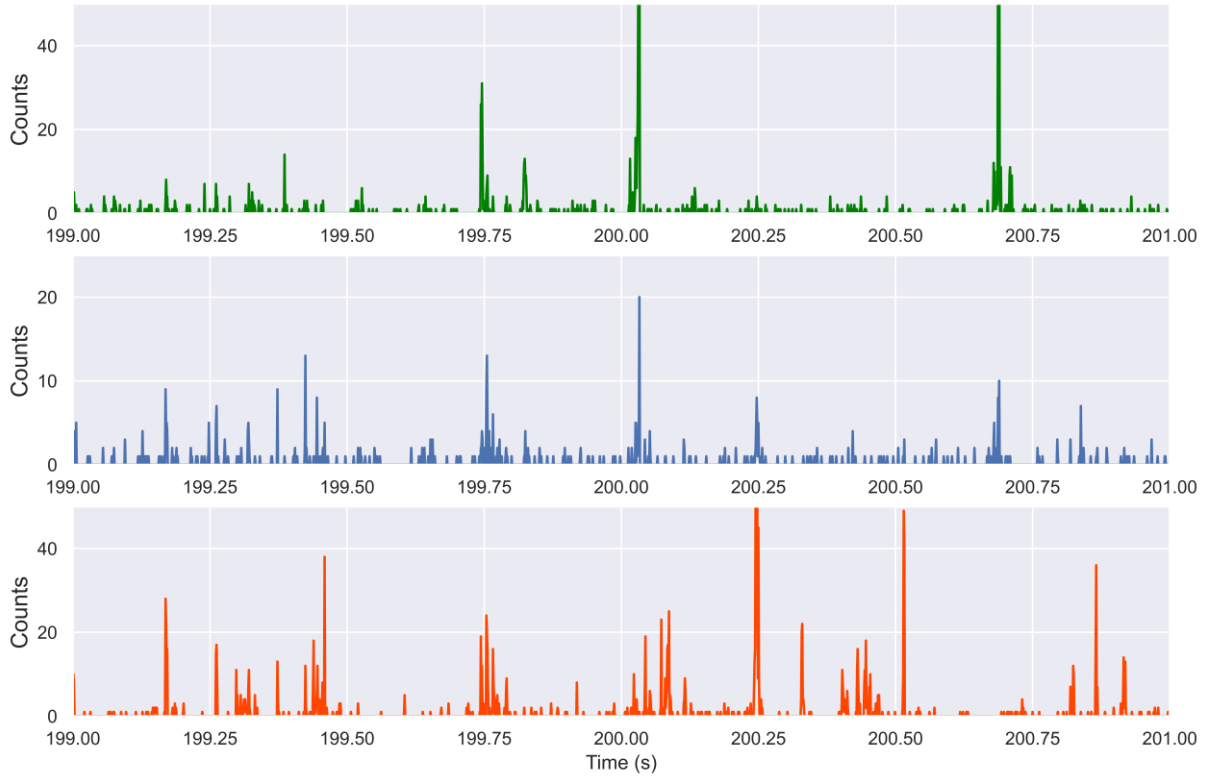
Figure 29: Time trace of FRET labelled \alpha S, the top panel is I_{DexDem} the middle panel is I_{DexAem} and the bottom panel is I_{AexAem} . A FRET burst occurs if there is a signal detected in all three time traces simultaneously, for example at t=199.75s . A donor-only burst occurs when only a signal at I_{DexDem} is detected, there is no example for this in the time trace. Leakage of donor signal to the acceptor channel can be detected by the presence of I_{DexDem} and I_{DexAem} while signal is absent at I_{AexAem} , for example at t=200.70s . An acceptor only burst occurs when only signal is detected at I_{AexAem} , for example at t=200.50s . Direct acceptor excitation occurs when a signal is detected at I_{DexAem} and I_{AexAem} while there is no signal at I_{DexDem} , for example at t=200.25s .
