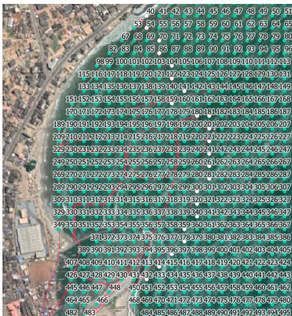
Figure 19: Elmina SWAN grid with breakwater outline (IMDC, 2021).
