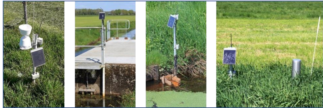
Figure 21 Examples of the four data collection station types. Left to right; precipitation and soil moisture content (groundwater gauging tube not visible); surface water level; drainage volume; groundwater level (soil moisture content probe not visible).
