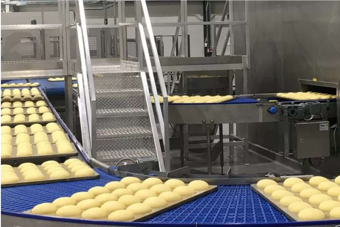
Figure 1: Peel boards carrying products on the production line along a conveyor belt (from Kaak website)
