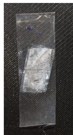
Figure 3.10: Etched piece, heated at 80 degrees exposed to UV light for 5 minutes.
