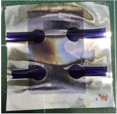
(a) The PVDF film with PDF attached, positive side/ front.
