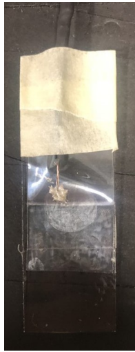
Figure 5.4: Transducer with circular ITO coating placed on glass slide
