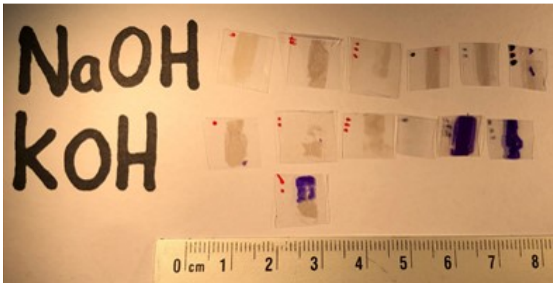
Figure 3.6: Etched films, PDF was removed with several concentrations NaOH and KOH. Color-coded films; red is type A, black is type B. 1 dot is 5%, 2 dots is 1% and 3 dots is 0.1% concentration. The ITO shape in the middle of the films is visible.
