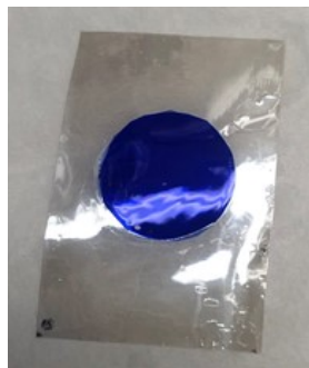
(b) PVDF with ITO coating and cured PDF, 80 degrees Celsius, 5 minutes in UV source.
