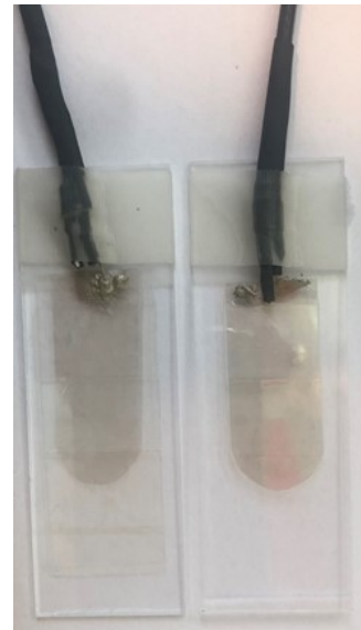
Figure 5.5: The transducers for testing the films properties. Processed film left and unprocessed film right.
