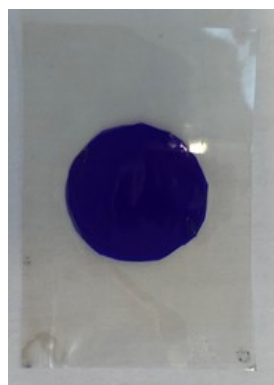
(c) PVDF with ITO coating removed.
