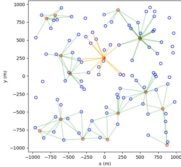
FIGURE 3: Adding a single base station when maximizing the average SNR considering  $60 \times 60$  possible positions.
