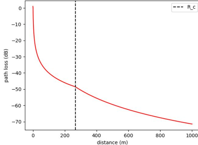
FIGURE 1: Dual slope path loss  $\ell_2(r_{ij})$  with a critical distance of  $267m$ .
