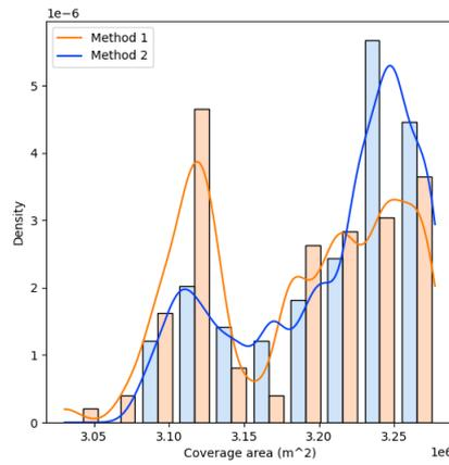
(b) Density plot of the coverage area of Method 1 against Method 2 for the standard graph with a reduced critical distance of 20%.
