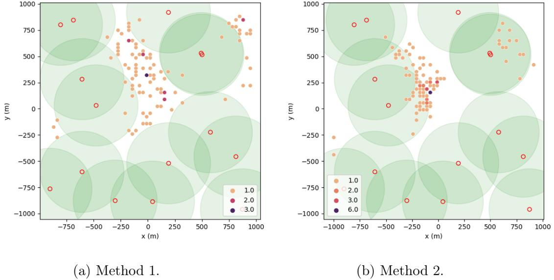
FIGURE 11: The positions of the users in the standard graph are simulated 100 times and the dots are the coordinates of the newly deployed base stations.
