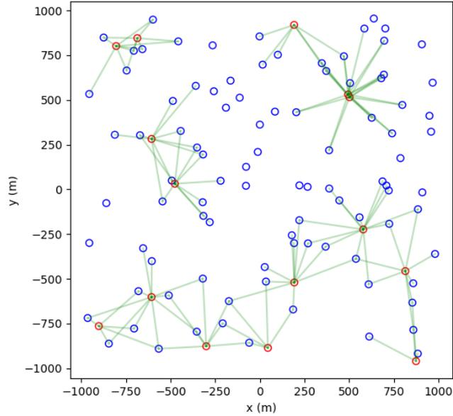
FIGURE 2: Standard graph of users and base stations. Base stations are red, users are blue and connections are green.
