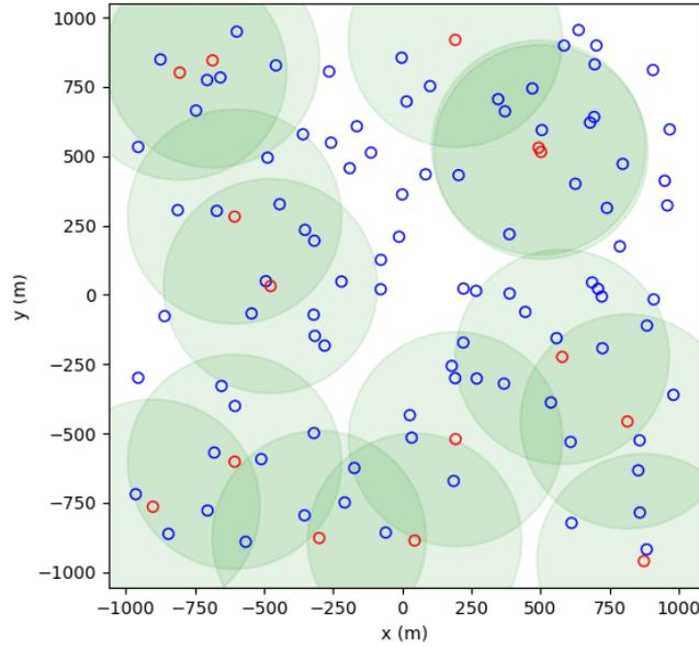
FIGURE 5: Coverage area of all base stations for a critical distance of 267 m.
