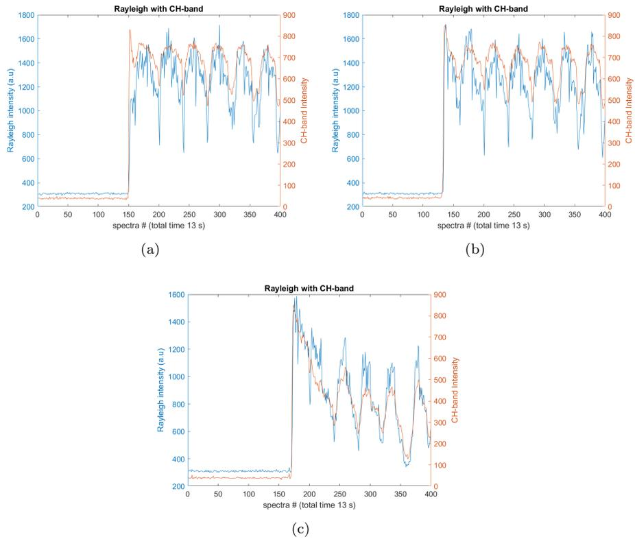
**Figure 13:** The Rayleigh intensity on the left y-axis in comparison CH-band on right axis over the spectra of one measurement. All the figures show oscillation in the trapping event for sample BN. The measurements were on 13-06-2022 (a) Measurement at 14:35:04 (b) Measurement at 14:35:26 (c) Measurement at 14:35:48
