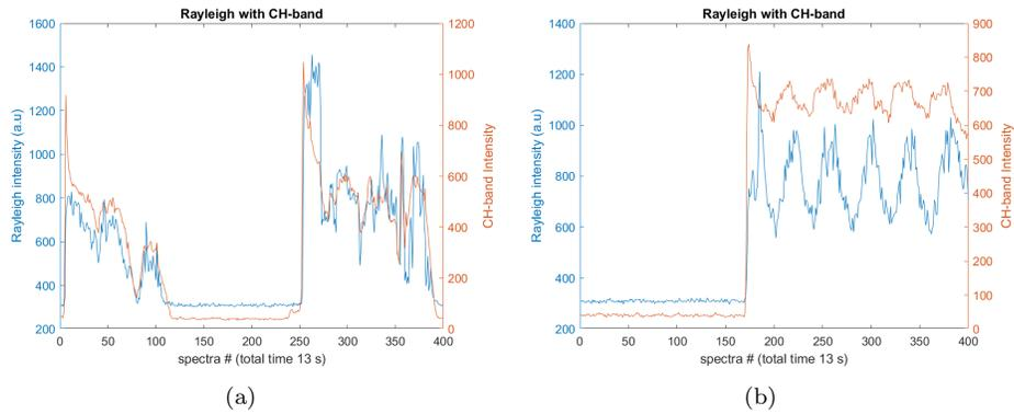
**Figure 12:** The Rayleigh intensity on the left y-axis in comparison CH-band on right axis over the spectra of one measurement. Both figures show an oscillation in the trapping event for sample AN . Both measurements were on 13-06-2022 (a) Measurement at 13:46:57 (b) Measurement at 13:47:42
