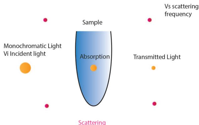
**Figure 2:** Raman principle: Incoming Monochromatic light with  $\nu_i$  (Incident frequency) goes through the sample. Some of the light is absorbed, the remaining light that leaves the sample is the transmitted light. From incident light some light is scattered. These are scattered with the scattering frequency  $\nu_s$
