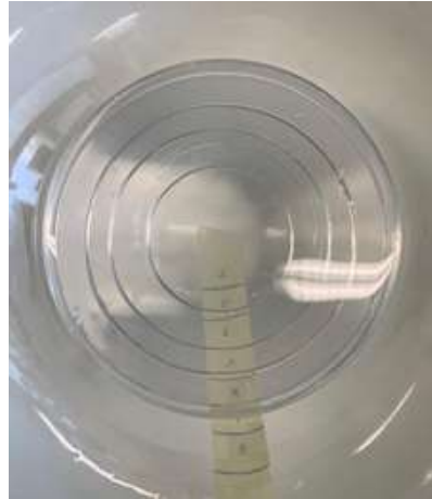
Figure C.2: Example of a PVC cup (top view) with marked tape to indicate the desired layer thickness. Example shown is a test version and not the final version used in the experiments.
