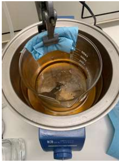
Figure C.1: The 2000 mL glass beaker is filled with native gel wax and placed in the oil bath of 150 °C. The gel wax inside the glass beaker was melted under regularly stirring with a metal spoon.
