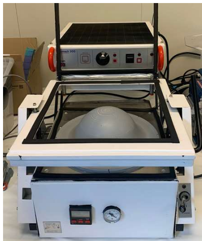
Figure A.2: Cup mould (size 8) placed in the vacuum shaping machine at PA imaging.
