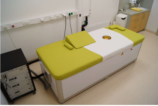
Figure 2.2: The PAMMOTH photoacoustic tomographic breast imager, positioned in the MST hospital in Oldenzaal.
