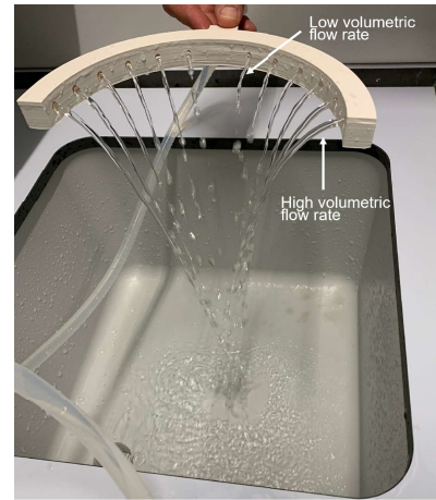
Figure 5.7: Image of the water supply ring being tested with water. The volumetric flow rate differed per hole size.
