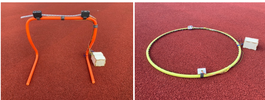
Figure 6.1: Realization of the slave module, consisting of distance sensors and an LED strip
