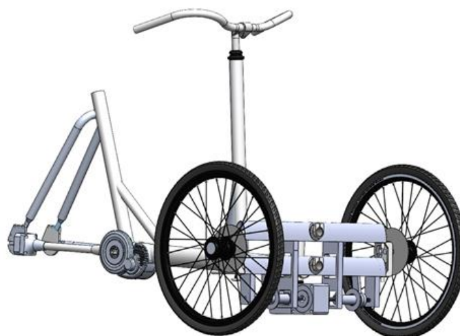
Figure 23 Final design of the trike with stabilizing mechanism.
