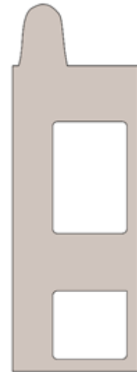
Figure 19 Connector with fixation to upper wheel axis and holes for the lower wheel axis and spindle.
