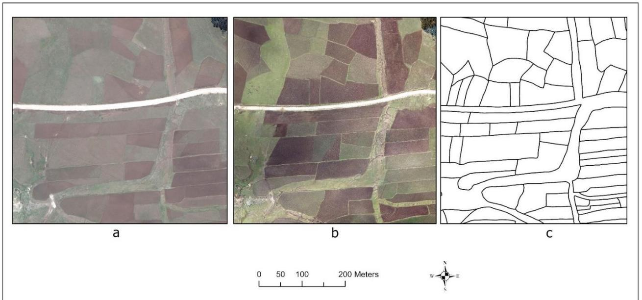
Figure 8: Snapshot of aerial (a) and UAV orthophoto (b) with corresponding cadastral boundaries (c)
