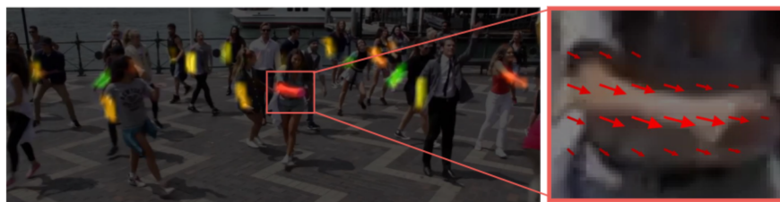
Figure A.6: The bottom-up approach using Part Affinity Fields to detect the limb [3]
