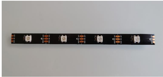
Figure 15: A strip of 4 WS2812b LED's
