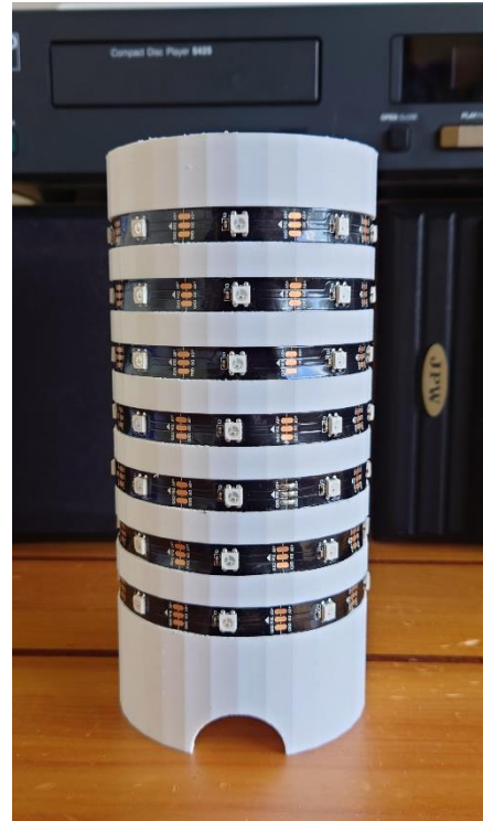
Figure 22b: Column with LED's installed
