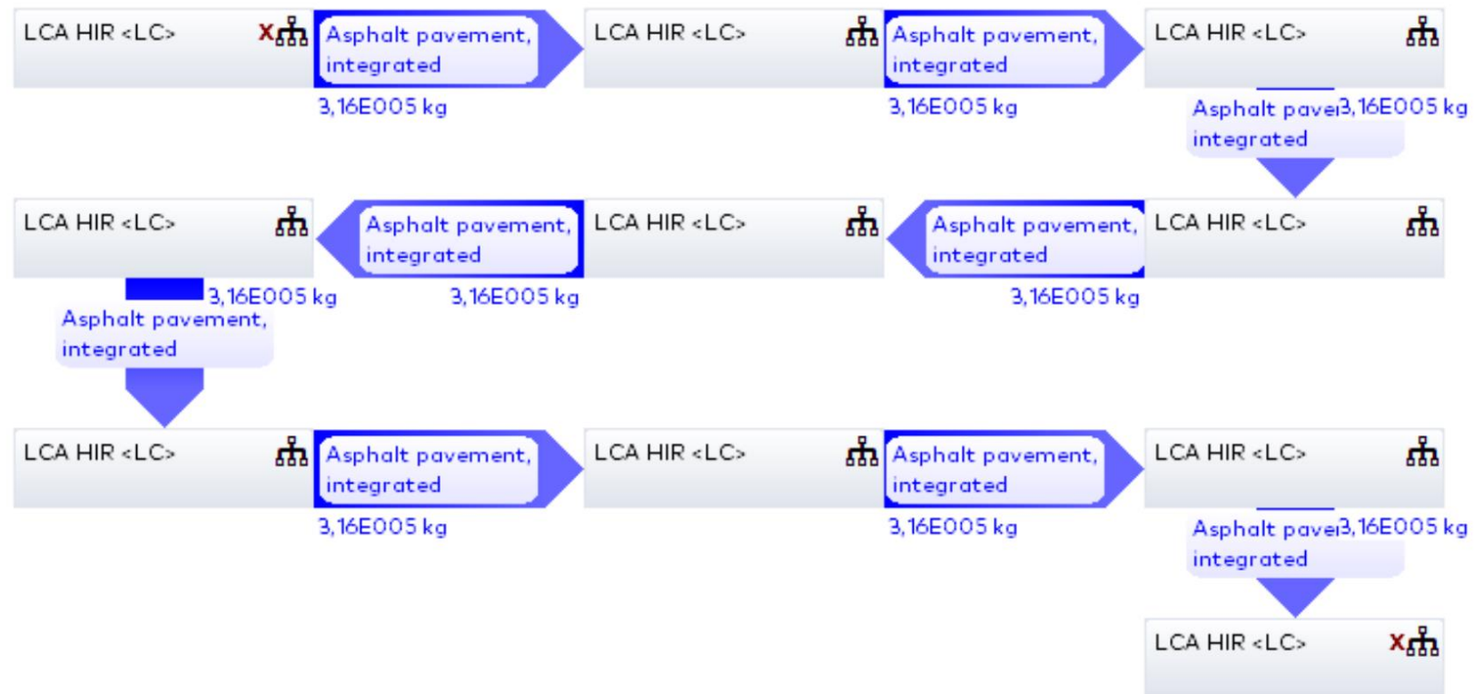
Figure 11 LCA Model of Hot In-place Recycling (HIR) for analysis period of 100 years (worst scenario-lifespan 10 years)
