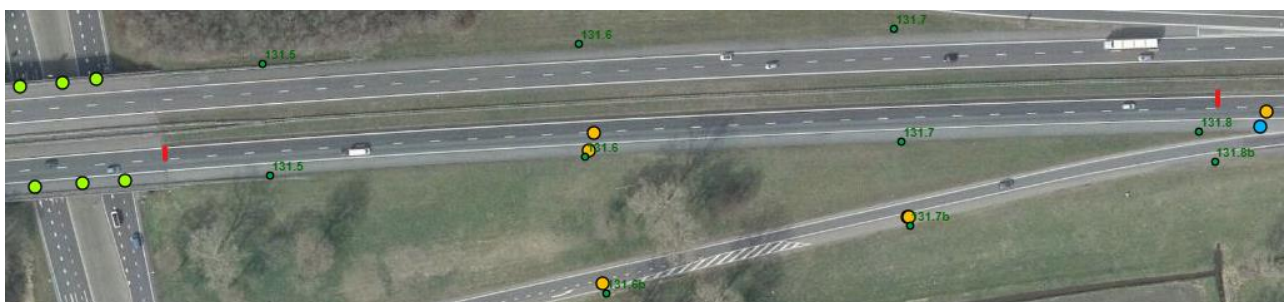
Figure 12: Drilling cores on a visually different top layer section. A1 100-meter marker 131.4 – 131.8 (Section of different color in between the red lines)
