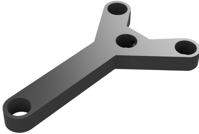
*Fig. 18: 3D model of aluminum PCB holder*
