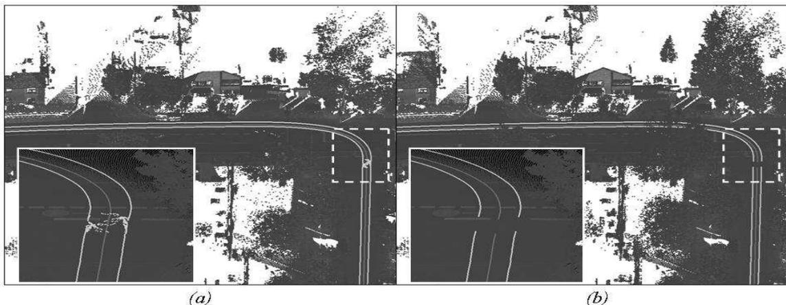
*Figure 4-7: Estimated sensor trajectory (a) without filtering stopping points and (b) after filtering*
