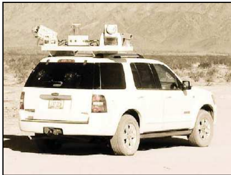
Figure 2-1. Vehicle based mobile laser scanning (Optech, 2008)
