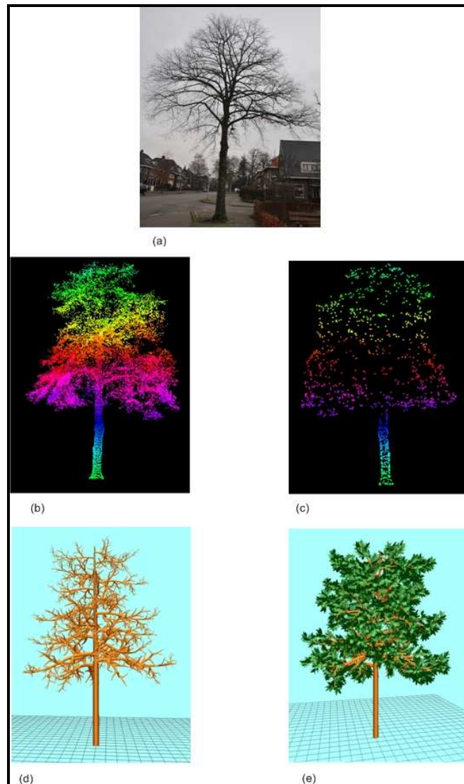
Figure 5-3. 3D tree model (a) Photo graph of tree, (b) mobile laser scan point cloud of tree (c) 3D alpha shape of tree (d) 3D model of the tree (e) Textured 3D tree model
