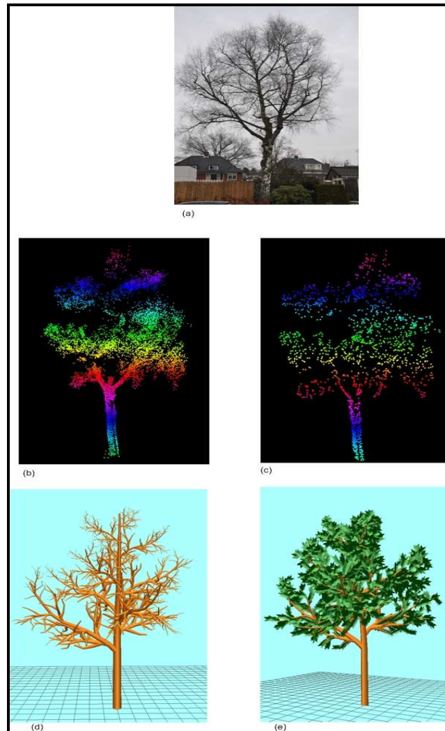
Figure 5-4. 3D tree model (a) Photo graph of tree, (b) mobile laser scan point cloud of tree (c) 3D alpha shape of tree (d) 3D model of the tree (e) Textured 3D tree model
