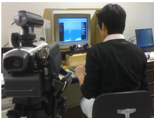
Figure 3.9: The applied faceLAB eye tracker running the stimulus. The user's monitor is captured via an external camera as back up.
