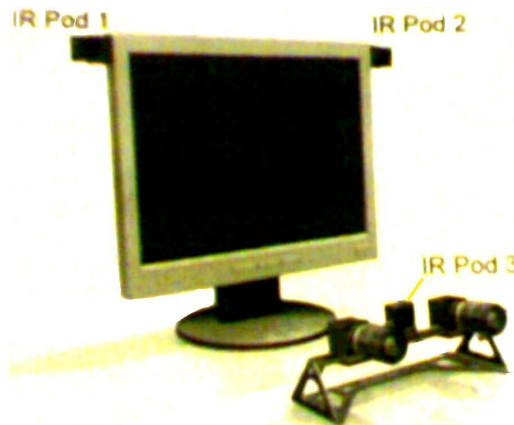
Figure 3.8: The faceLAB eye tracker with a pair of Flea cameras and three IR pods.
