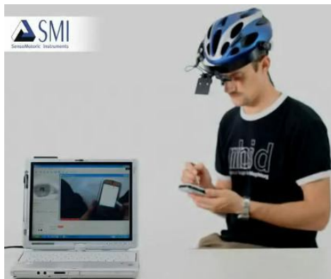
Figure 3.3: Illustration of the usual use of a mobile eye tracker (SMI iView) for the PDA inspection, while the user is in a stationary state. The user's field of view can be observed on line, by the related software. It can be noticed that the field of view (even without any lens) is small and if the user moves his hand a little, the PDA falls out of the camera view field (URL_8).
