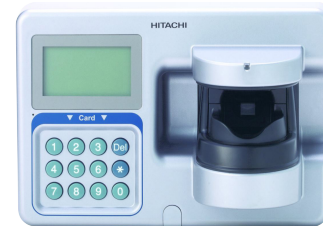
Fig. 1: Hitachi SecuaVeinAttestor authentication terminal [7]
