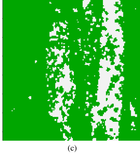
Figure 5.17: (a) SVM classified image. (b) MRF-SVM classified image with \lambda = 0.85 . (c) MRF-MLC classification results with \lambda = 0.95 .
