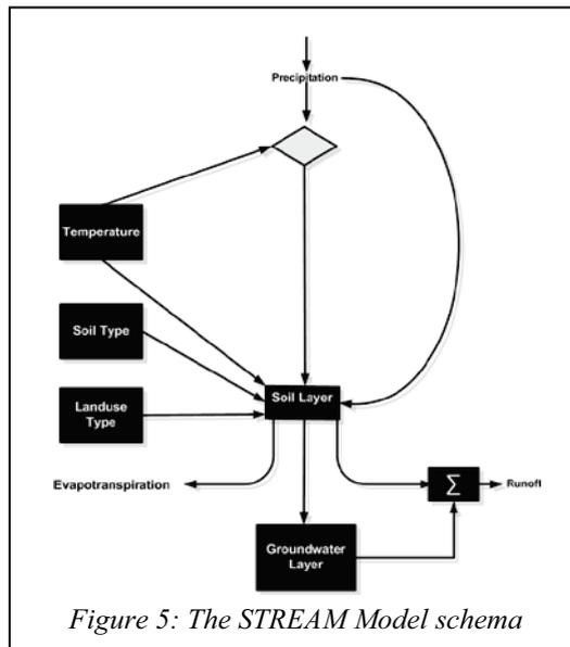
Figure 5: The STREAM Model schema
