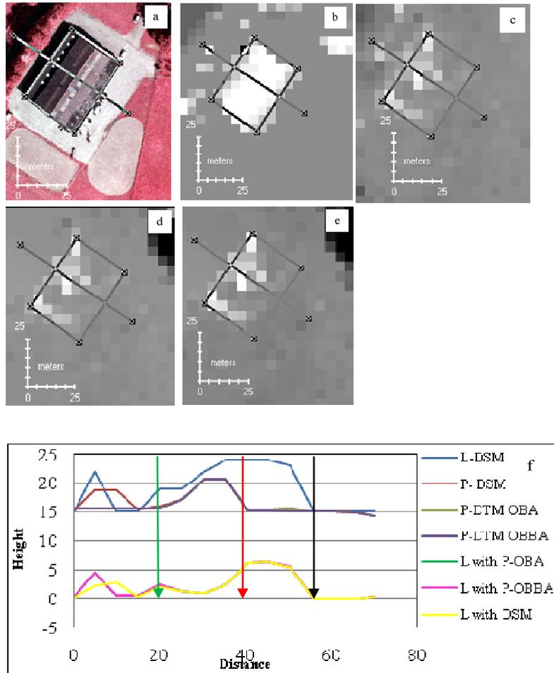
**Figure 4.17:** Accuracy assessment of single house (a) orthophoto (b) LIDAR DSM (c) Photogrammetric DSM (d) Pseudo-DTM with OBA (e) Pseudo-DTM with OBBA (f) spatial profile of height and standard deviation (with respect to L-DSM) along the transects seen in pictures.
