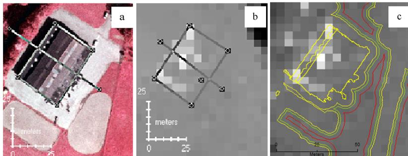
**Figure 4.7:** Application of the normal buffer and the OBB approach on data set II (a) orthophoto representation (b) result from OBB and normal buffer method (same result) (c) Extent of DSM that would be removed by different width of buffer (Table 3.3).
