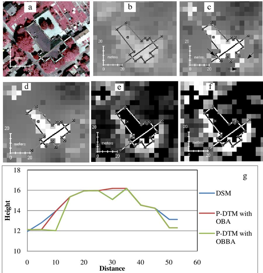
**Figure 4.13:** Representation of house along with tree and shadow( a) outline of house in orthophoto (b) representation in DSM (c) Pseudo-DTM with OBA (d)Pseudo-DTM with OBBA (e)difference from OBA (f) difference from OBBA(g) spatial profile along the transects indicated in pictures.
