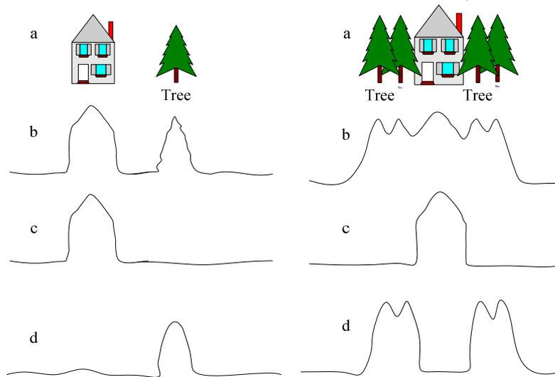
**Figure 3.7:** Schematic representation of features and their profile in DSM (a) photograph b) LIDAR DSM c) Pseudo-DTM d) standard deviation between the LIDAR and Pseudo-DTM.
