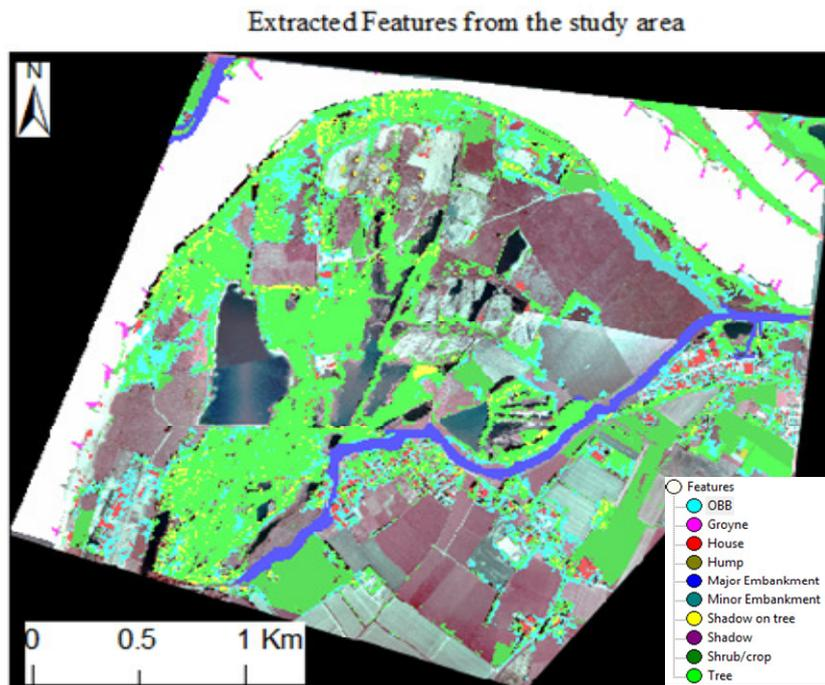
**Figure 8.7:** *Extracted image showing the objects that have been considered under the study. Includes the features that are not removed from the DSM.*
