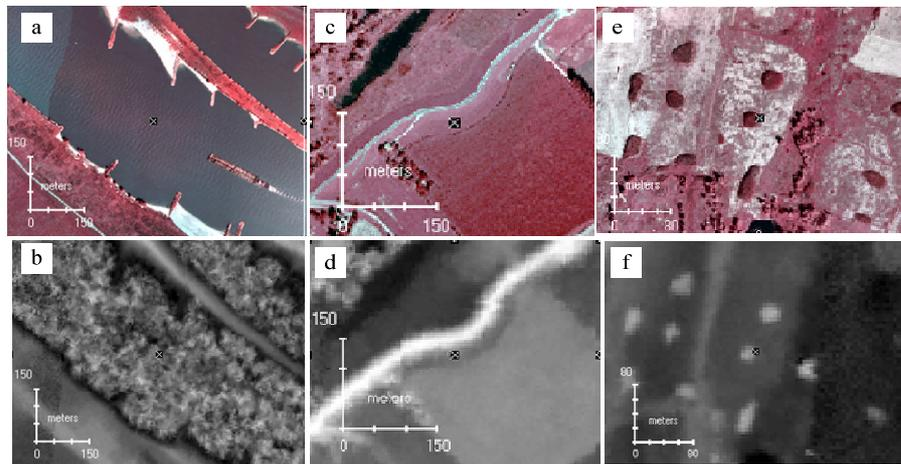
**Figure 8.4:** Groyne representation-(a, b), Embankment representation-(c, d) Hump representation-(e, f)
