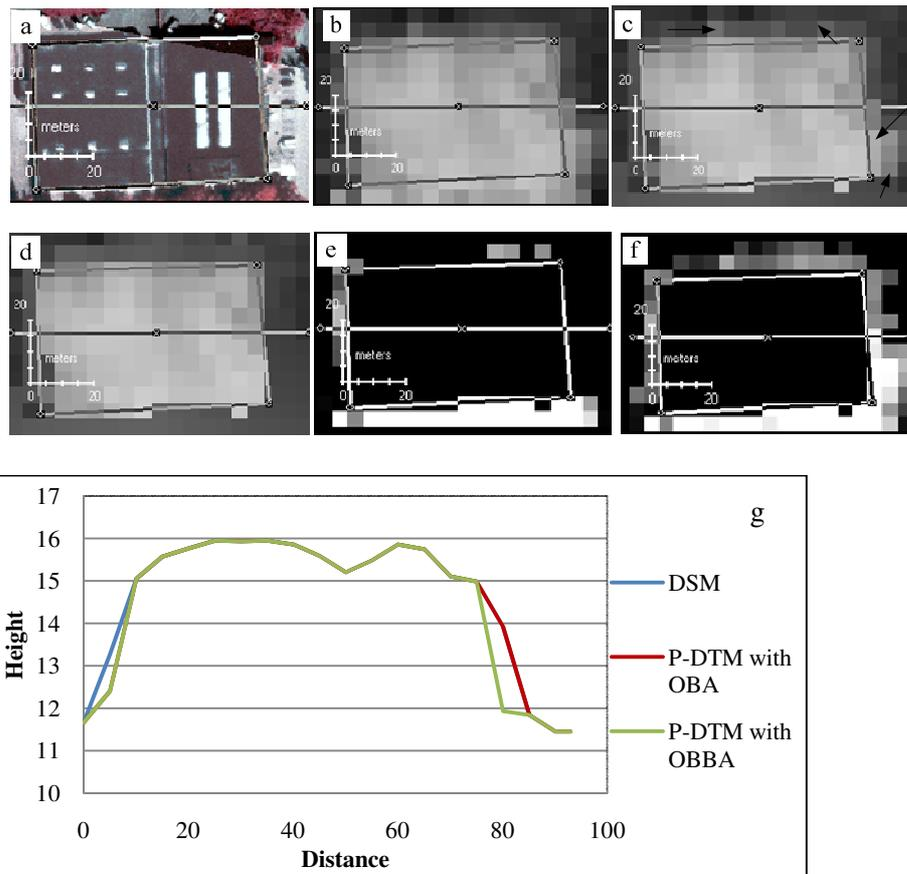
**Figure 4.10:** Single house and its representation (case II) (a) outline in orthophoto (b) DSM (c) Pseudo-DTM with OBA (d) Pseudo-DTM with OBBA (e) difference from OBA (f) difference from OBBA (g) spatial profile along the transects seen in images.
