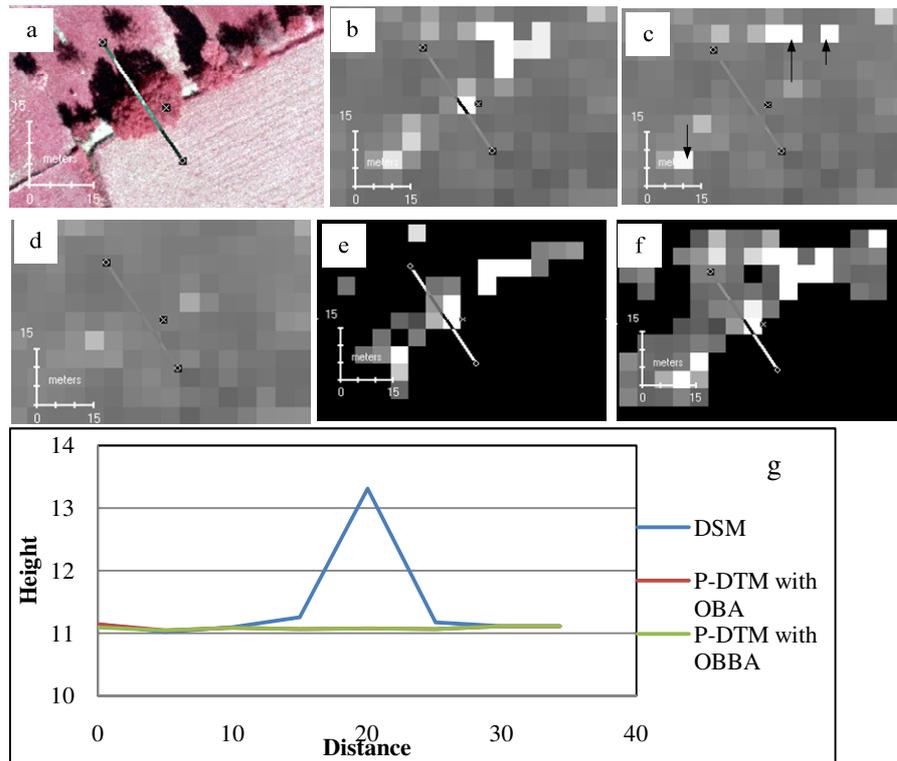
**Figure 4.8:** Single tree representation (a) orthophoto (b) DSM (c) Pseudo-DTM with OBA (d) Pseudo-DTM with OBBA (e) difference of OBA (f) with OBBA (g) spatial profile along the transects seen in pictures.
