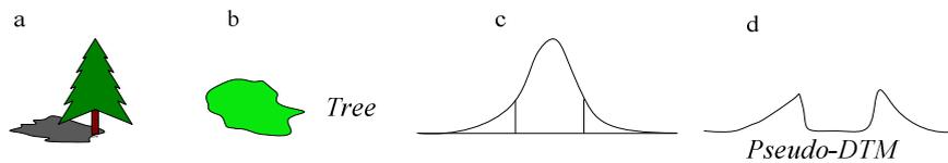
**Figure 3.5:** Schematic representation of the feature removal by OBA approach; (a) tree along with shadow, (b) identified tree, (c) area in DSM defined by identified tree and (d) Pseudo-DTM.
