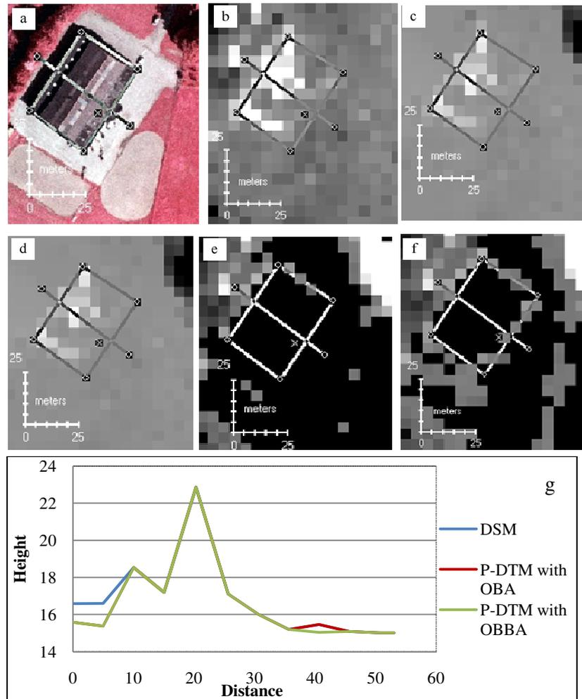
**Figure 4.9:** Single house and its representation (case I) (a) outline in orthophoto (b) DSM (c) Pseudo-DTM with OBA (d) Pseudo-DTM with OBBA (e) difference from OBA (f) difference from OBBA (g) spatial profile along the transects seen in pictures.
