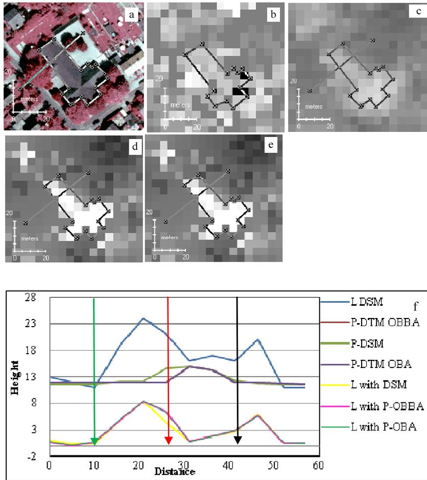
**Figure 4.20:** Accuracy assessment of compound case I, representation on (a) orthophoto (b) L DSM (c) P-DSM (d) Pseudo-DTM with OBA (e) Pseudo-DTM with OBBA (f) spatial profile of height and standard deviation (with respect to L-DSM) along the transects seen in pictures.
