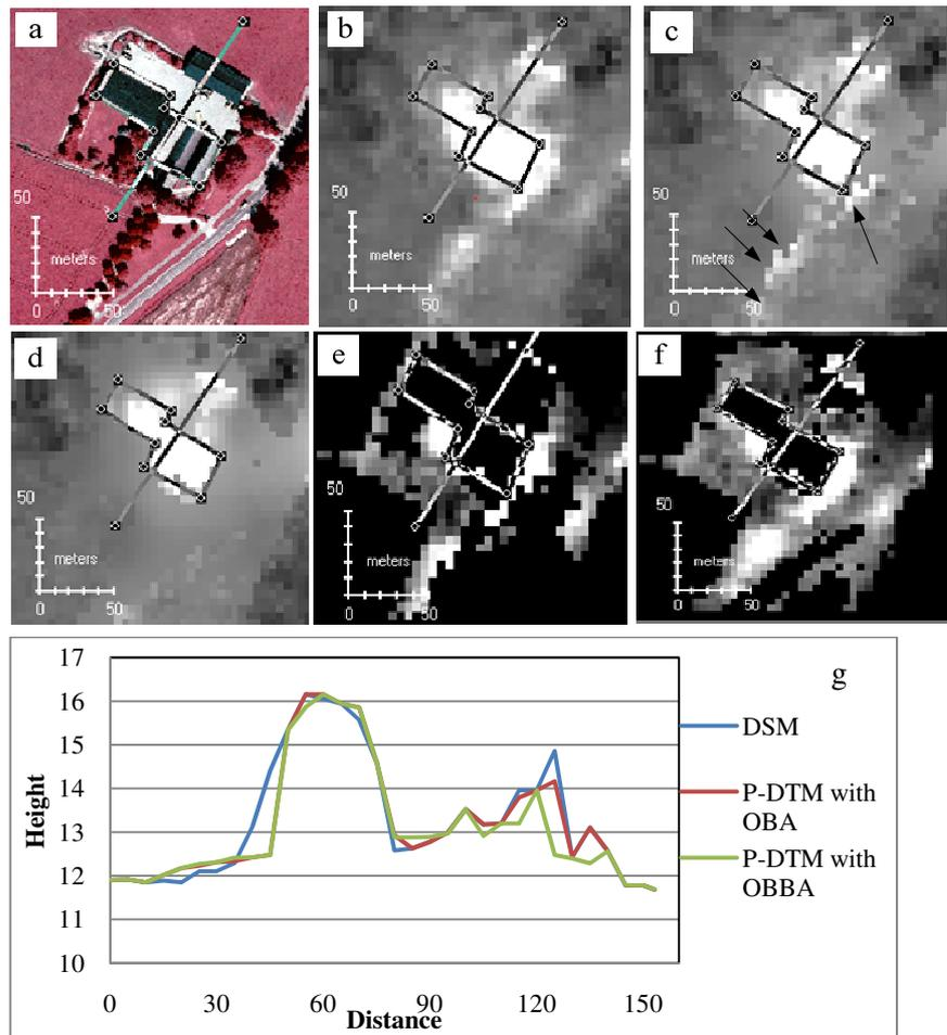
**Figure 4.14:** Representation of house along with tree and shadow( a) outline of house in orthophoto (b) representation in DSM (c) Pseudo-DTM with OBA (d)Pseudo-DTM with OBBA (e)difference from OBA (f) difference from OBBA(g) spatial profile along the transects indicated in pictures.
