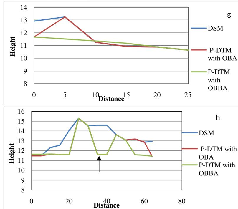
**Figure 4.15:** Representation of house along with tree and shadow (a) outline of house in orthophoto (b) representation in DSM (c) Pseudo-DTM with OBA (d)Pseudo-DTM with OBBA (e)difference from OBA (f) difference from OBBA(g) spatial profile along the shadow as seen in (h)Spatial profile along the transects seen in pictures.
