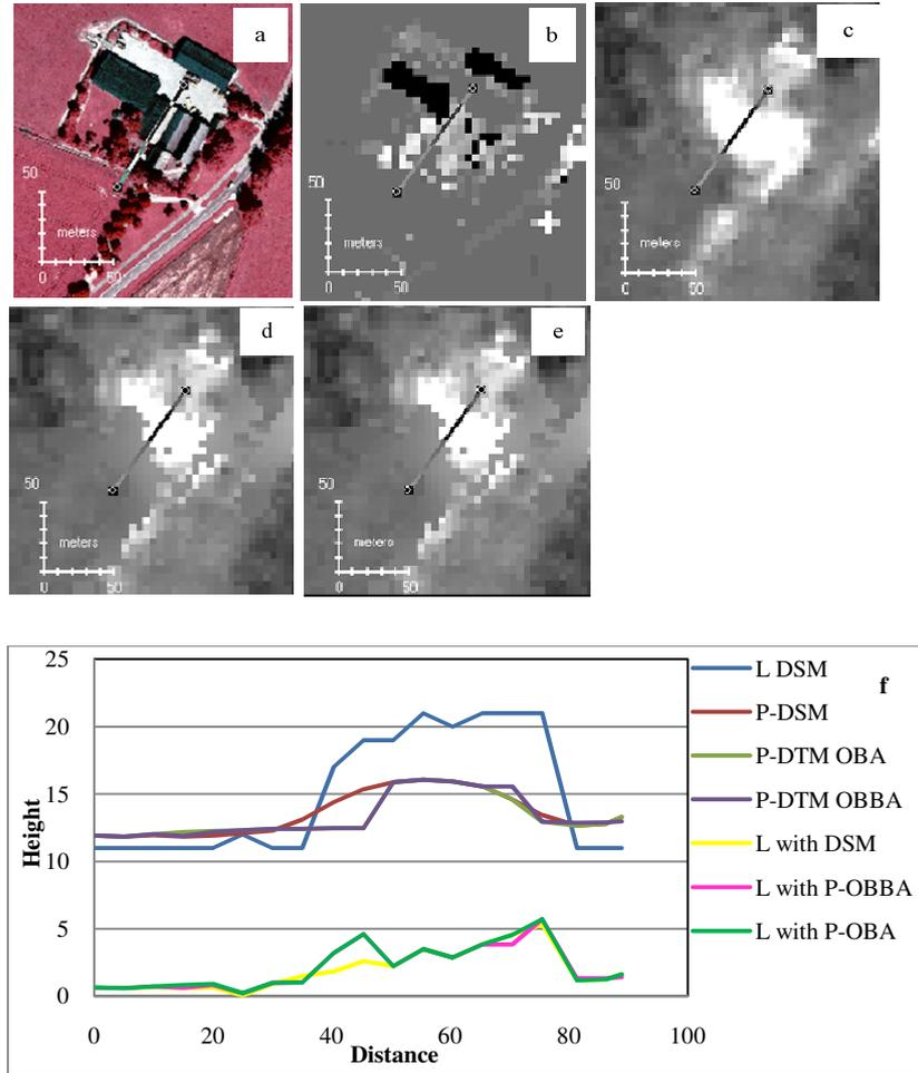
**Figure 4.21:** Accuracy assessment of compound case II, representation on (a) orthophoto (b) L-DSM (c) P-DSM (d) Pseudo-DTM with OBA (e) Pseudo-DTM with OBBA (f) spatial profile of height values along with standard deviation with respect to L-DSM along the transects as seen in pictures.
