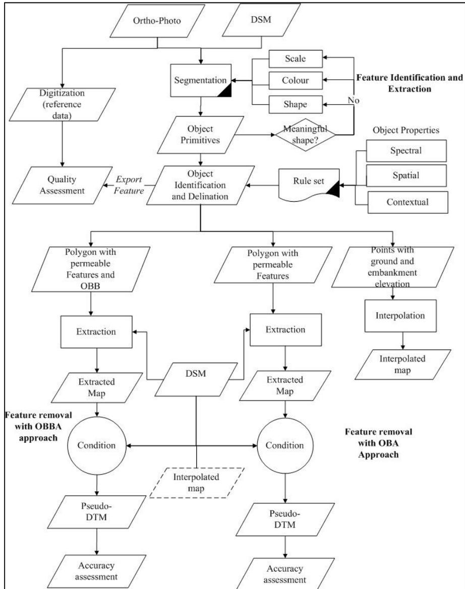
**Figure 3.8:** Work flow of proposed method for identifying and removing features from DSM
