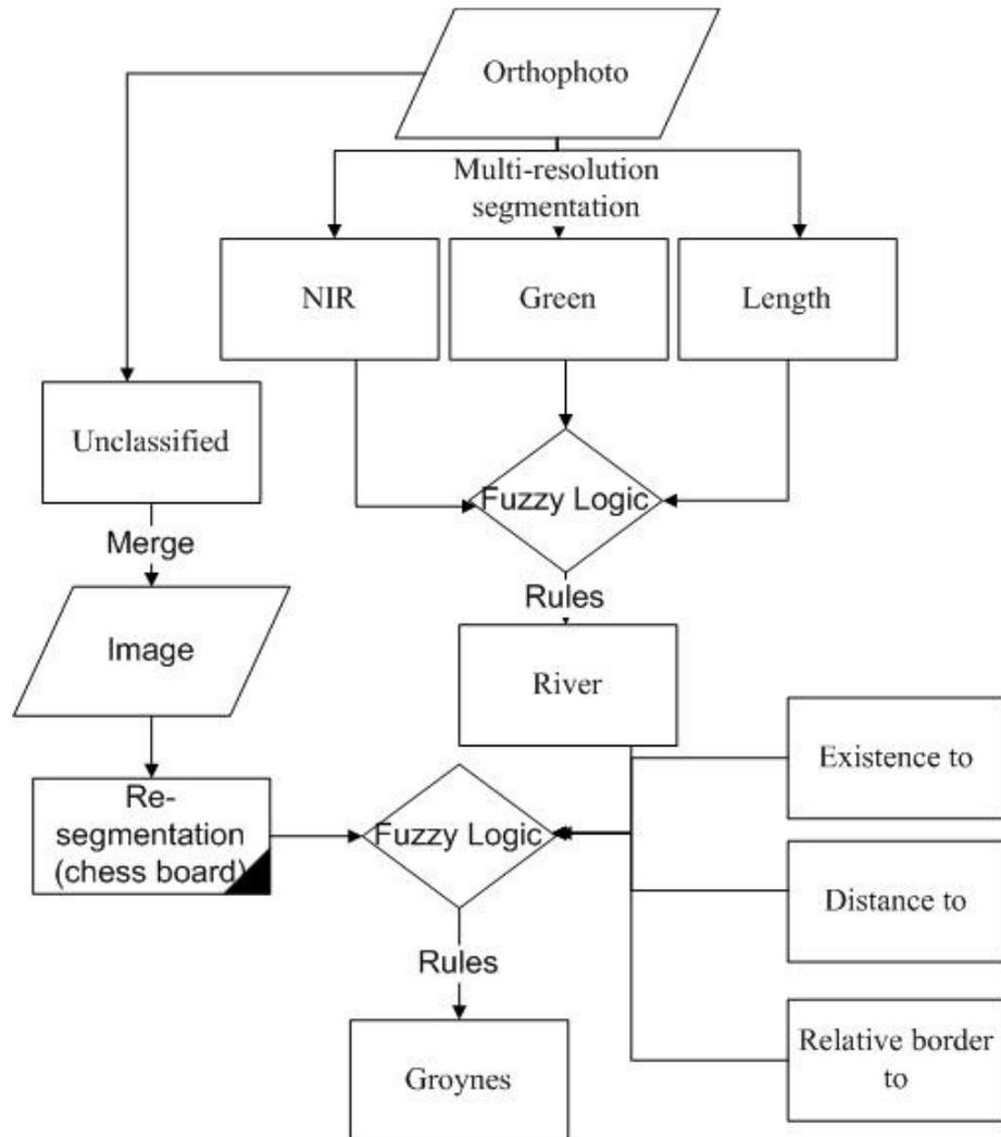
**Figure 8.6:** An example on identification and delineation of features. Groyne are separated from the image using two different level of segmentation and rule set that combines various spectral and contextual properties of features.
