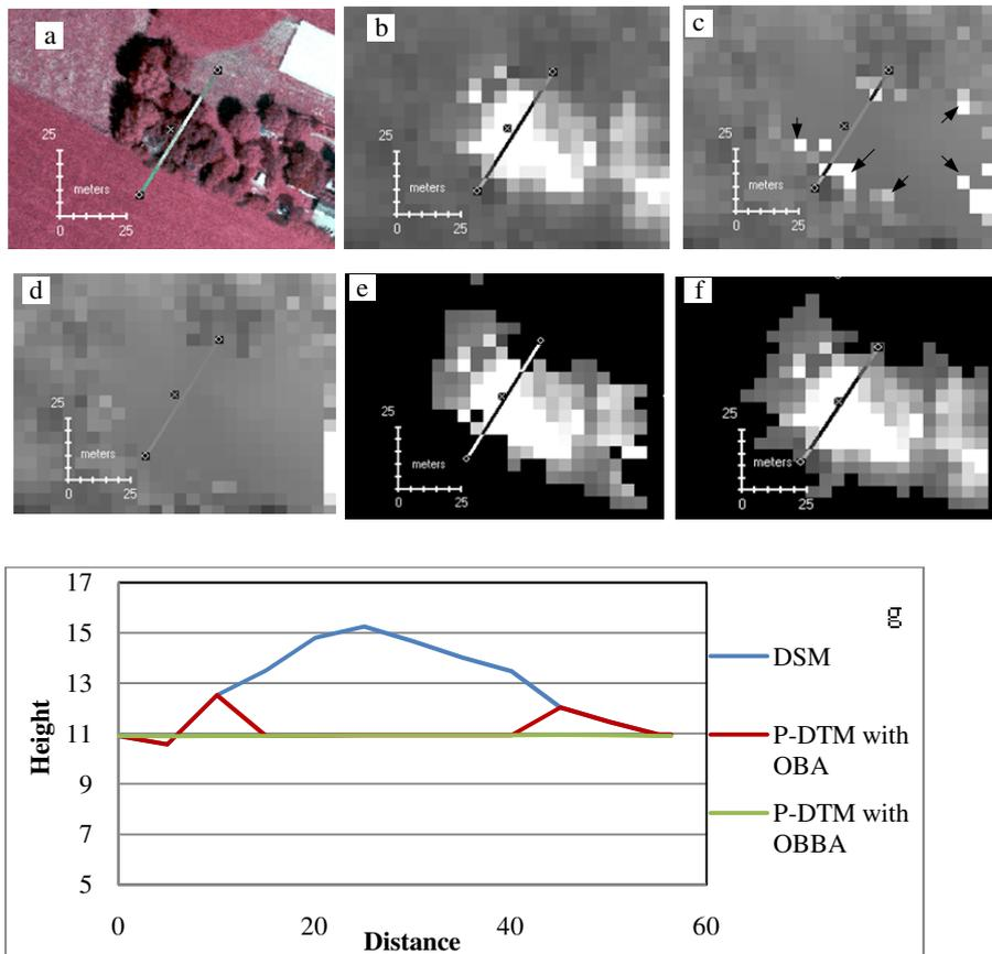
**Figure 4.11:** Tree clump and its representation (Case I) (a) orthophoto (b) DSM (c) Pseudo-DTM with OBA (d) Pseudo-DTM with OBBA (e) difference from OBA (f) difference from OBBA (g) spatial profile along the transects seen on pictures.
