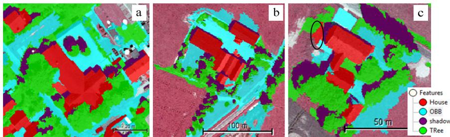
**Figure 4.4:** Identification and delineation of compound case houses (a) case I (b) case II (c) case III.
