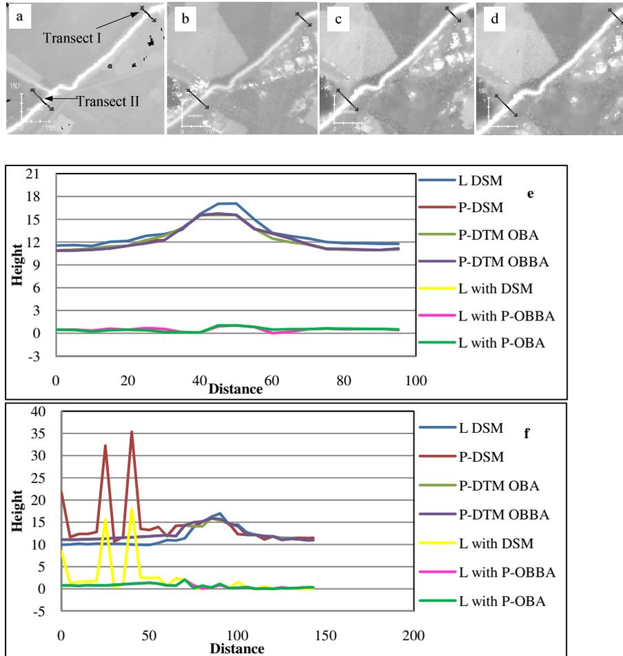
**Figure 4.19:** Profiles along the transects I and II on (a) LIDAR DTM, (b) Photogrammetric DSM, (c) Pseudo-DTM with OBA, (d) Pseudo-DTM with OBBA (e) Profile along transect I and (f) profile along transect II as seen in pictures.
