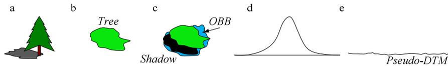
**Figure 3.6:** Schematic representation of the feature removal by OBBA approach; (a) picture (b) identified tree and shadow (c) Identified tree with OBB (d) DSM representation of the tree (e) Pseudo-DTM after application of OBBA approach.
