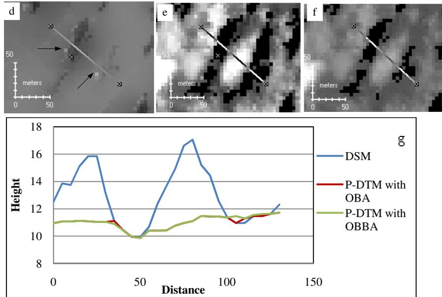
**Figure 4.12:** Tree clump and its representation (a) orthophoto (b) DSM (c) Pseudo-DTM with OBA (d) with OBBA (e) difference from OBA (f) difference from OBBA approach (g) spatial profile along the transects indicated in pictures.
