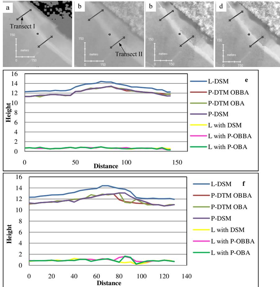
**Figure 4.18:** Profiles along the transects I and II on a) LIDAR DTM, (b) Photogrammetric DSM, (c) Pseudo-DTM with OBA, (d) Pseudo-DTM with OBBA, (e) Profile along transect I and (f) profile along transect II as seen in pictures.
