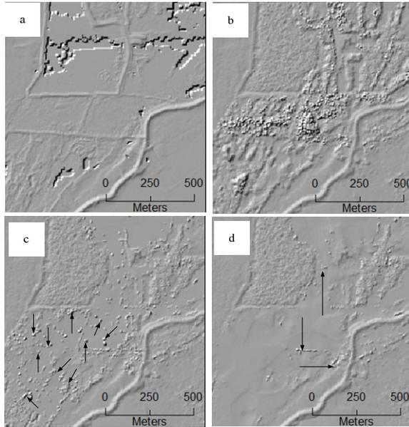
**Figure 4.16:** Hill shade analysis (a) LIDAR DTM (b) photogrammetric DSM (c) Pseudo-DTM created with OBA (d) Pseudo-DTM with OBBA.
