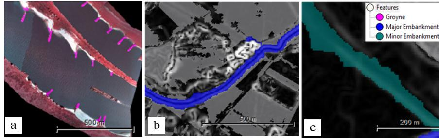
**Figure 4.3:** Identification and delineation of (a) groynes (b) major embankment (c) minor embankment.
