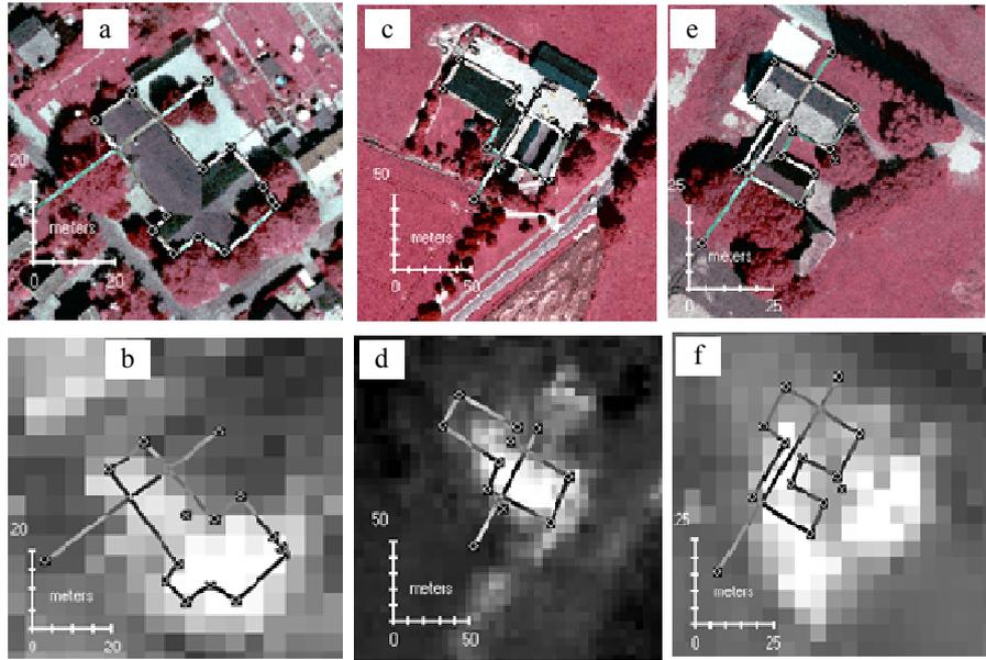
**Figure 8.5:** House representation in orthophoto and DSM; Case I (a, b), Case II (c, d) Case III (e, f)
