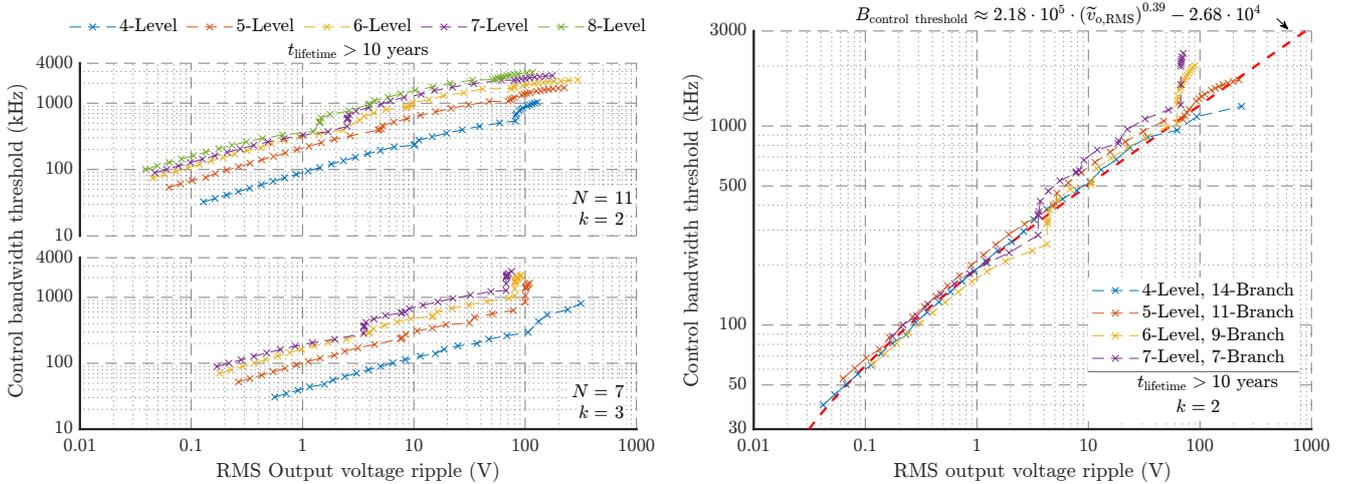
Fig. 15. Trade-off between RMS output voltage ripple and control bandwidth, showing how, independent of the exact number of levels and branches, an FCC with a larger output ripple has a larger potential control bandwidth given an effective switching frequency.
