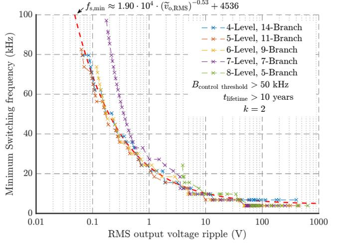
(b) FCC designs with a varying number of levels and branches such that the frequency doubling effect is approximately consistent across the different number of levels. Showing how the relationship between switching frequency and output voltage ripple is not necessarily dependent on the number of branches and levels but rather on the effective switching frequency, a combination of the two.
