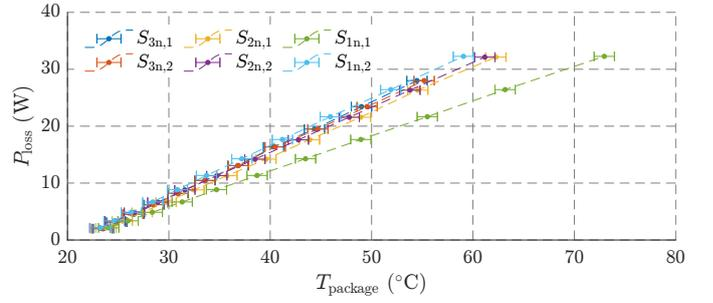
Fig. 22. Mapping from measured steady-state package temperature to losses for the 6 listed FETs, shown with temperature measurement error. Most FETs show the same behavior with only  $S_{1\text{n},1}$  reading a significantly higher package temperature.
