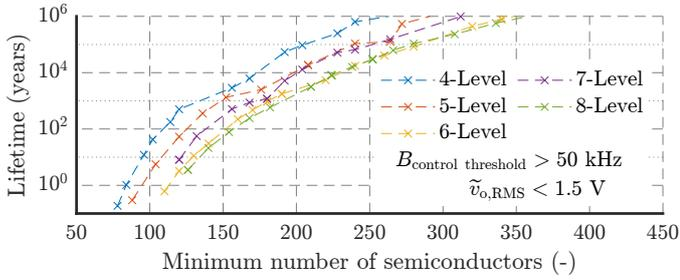
Fig. 19. Relationship between the minimum number of semiconductors  $2(M-1) \cdot N \cdot k$  and lifetime, showing how a longer lifetime requires more semiconductors, and how having more levels also increases the minimum semiconductor count for a given lifetime.
