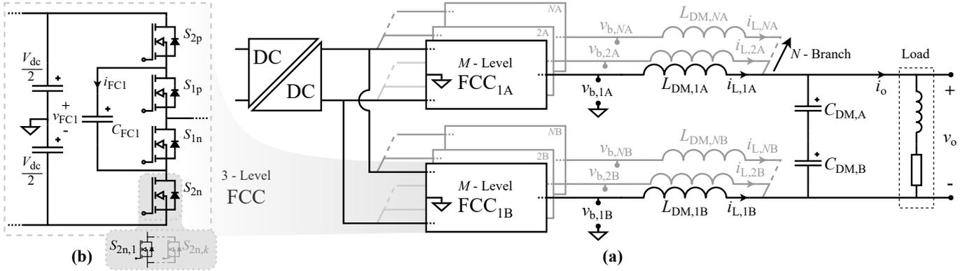
Fig. 1. a) FCC-based gradient amplifier topology with  $N$  parallel branches that each contain an  $M$ -level FCC cell. b) Example of a  $M = 3$  level FCC cell where 'k' indicates the number of parallel FETs per switching element.
