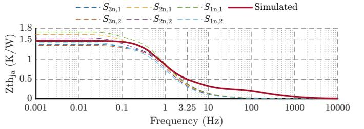
Fig. 26. Comparison between measured and simulated thermal impedance. The measurement was done at  $3.25\text{ Hz}$ , meaning any effects faster than that were not able to be captured. Up until this point, the measured impedance matches the simulated impedance closely.
