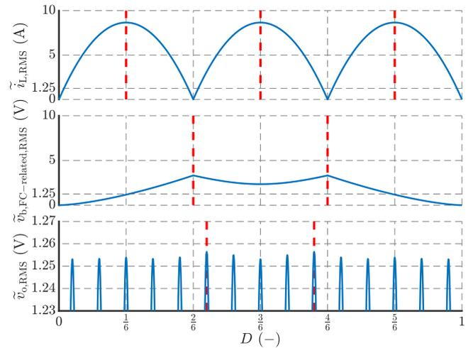
Fig. 5. Inductor current ripple (top), FC-related branch voltage ripple (middle), and output voltage ripple (bottom) as functions of duty-cycle of a 4-Level 5-Branch FCC. The red dashed lines indicate the worst-case operating points for each of the components. Note that the Y-axis is zoomed in for the bottom plot to make the difference in peak height visible.
