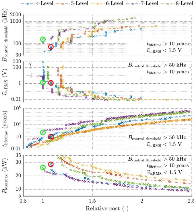
Fig. 16. Influence of cost on control bandwidth,  $B_{\text{control}}$  threshold, RMS output voltage ripple,  $\tilde{v}_{o,\text{RMS}}$ , lifetime,  $t_{\text{lifetime}}$ , and total loss,  $P_{\text{loss,max}}$ . Two designs have been marked with a circle, the lowest cost 4-Level and 7-level designs that satisfy all default constraints (24), also visible in the bottom plot. In most cases, the 7-level design has the best result for the lowest cost.
