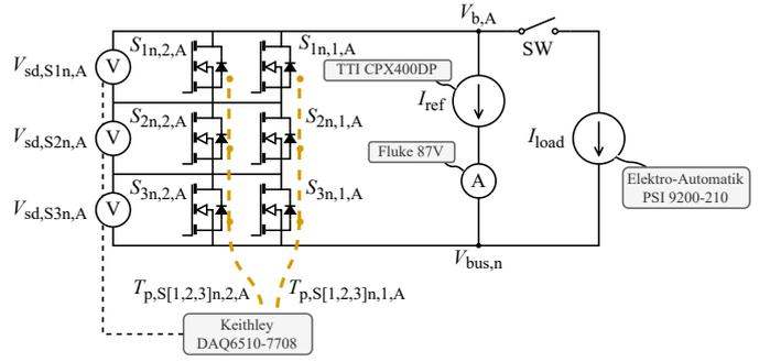
Fig. 25. Schematic measurement setup used to estimate the thermal impedance of the prototype. During the calibration of the  $V_{sd}$ ,  $T_j$  curve, SW is kept open. To heat the FETs, SW is closed and  $I_{load}$  is applied, afterwards, SW is opened again and  $V_{sd}$  is continuously measured to extract the cooldown curve.
