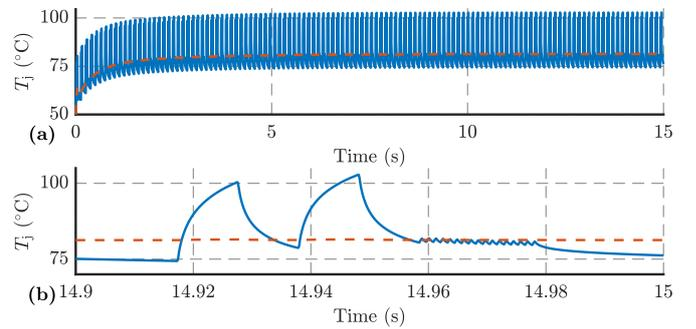
Fig. 9. Thermal response of junction temperature to the worst-case profile from **Fig. 6**: (a) Junction temperature in blue and its moving average in dashed orange over the entire 15 s. (b) Zoomed-in version showing just the final run of the profile, used for extracting the peak-to-peak and average junction temperatures.
