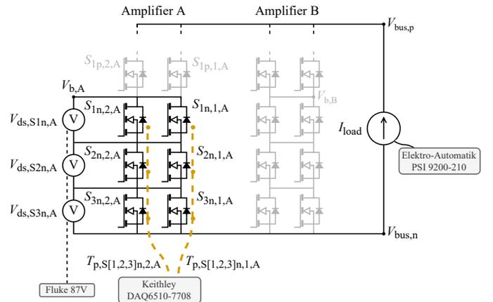
Fig. 21. Measurement setup used to measure the  $T_p$ ,  $P_{loss}$  relation from **Fig. 22**.
