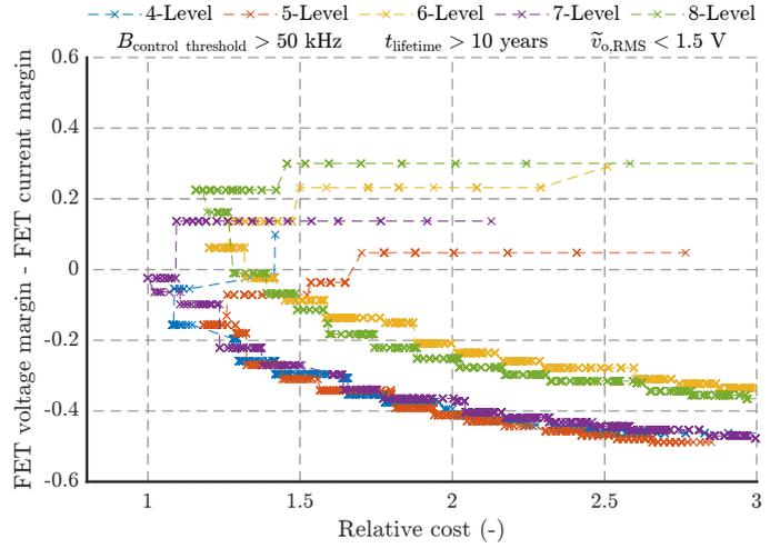
Fig. 18. Difference between FET voltage margin and FET current margin as a function of relative cost. Negative values imply a larger current margin while positive values imply a larger voltage margin. The most optimal design has approximately equal valued margins. Independent of the number of levels, the most optimal designs are always in the range  $-20\%$  to  $20\%$ .
