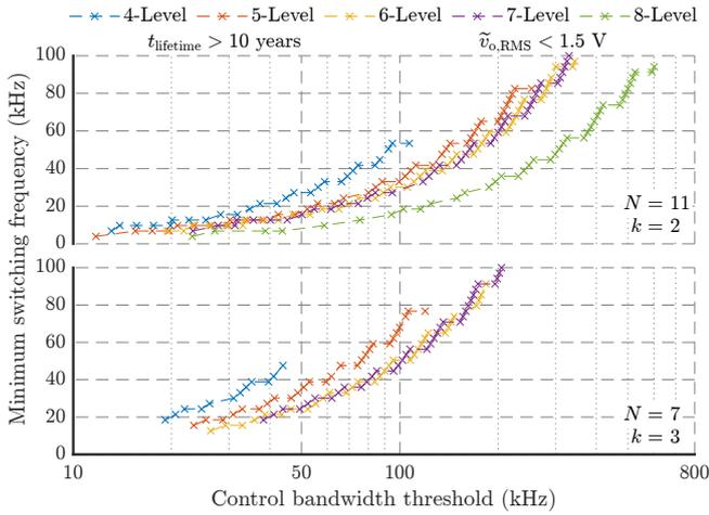
(a)  $M = 4, \dots, 8$ -Level FCCs with  $N = 11$  Branches and  $k = 2$  parallel FETs (top) and  $N = 7$  Branches and  $k = 3$  parallel FETs (bottom).
