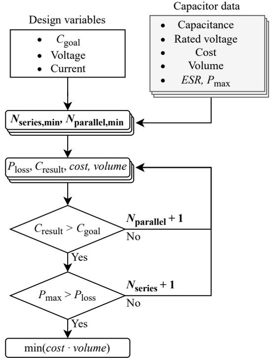
Fig. 10. Implemented capacitor design workflow for flying- and filter capacitors.
