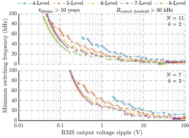
(a)  $M = 4, \dots, 8$ -Level FCCs with  $N = 11$  Branches and  $k = 2$  parallel FETs (top) and  $N = 7$  Branches and  $k = 3$  parallel FETs (bottom) showing similar results to Fig. 11.
