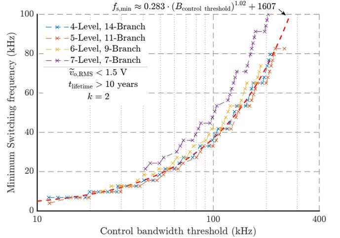
(b) FCC designs with a varying number of levels and branches such that the frequency doubling effect is approximately consistent across the different number of levels.
