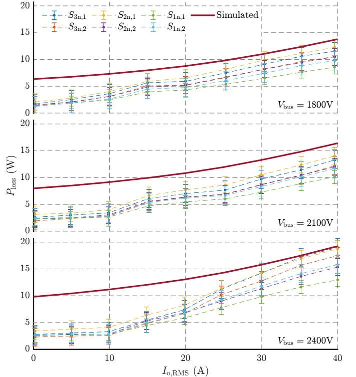
Fig. 24. Comparison between extracted and simulated steady-state loss (switching + conduction) at various RMS output currents and three bus voltages. The simulations always predict a higher loss than measured, matching more closely at higher output currents. The error margin, due to the temperature measurement error of both the calibration and this steady state measurement combined, is also shown in the form of error bars.
