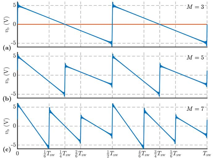
Fig. 4. Branch voltage  $v_b$  over time of a  $M = [3, 5, 7]$ -level FCC operating at  $D = 0.5$  to show only the FC related ripple  $\tilde{v}_{b,FC-related}$ : (a)  $C_{FC1} = \text{Inf}$  (orange) and (a,b,c) properly dimensioned  $C_{FCi}$  (blue) such that  $V_{b,FC-related,pp,max} = 10$  V. Gibbs phenomenon is not smoothed out.
