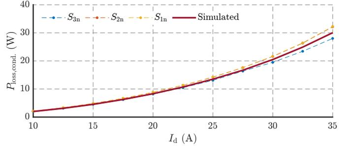
Fig. 23. Comparison between measured and simulated steady-state conduction loss at various drain currents, showing a clear match.
