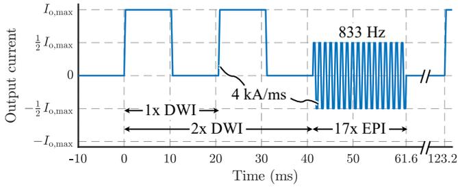
Fig. 6. Worst-case output current load profile consisting of 2 unipolar DWI pulses followed by 17 bipolar EPI pulses. 1 DWI pulse is approximately equal in length to the 17 EPI pulses. Following this 61.6 ms sequence is an equally long idle period. The profile repeats every 123.2 ms
