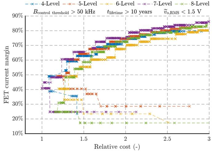
Fig. 17. FET current margin as a function of relative cost, showing that ideally, the current margin is between 40% and 50%, independent of the number of levels. The 8-level designs are the only exception due to their relatively high FET voltage margin.
