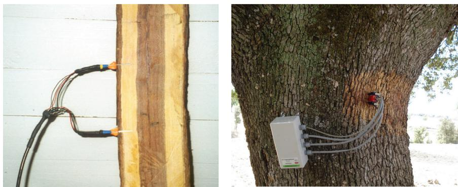
**Figure 4** Granier and HFD probes inserted into oak stems. The sensors were later protected from the sun and animals with stereopor and wire nets (picture of Granier sensors from Mapanda (2003)).
