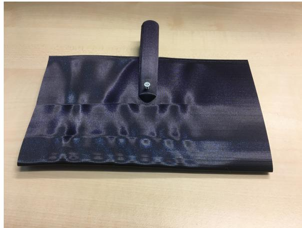
**Figure 4.2:** Warped airfoil after being placed under a halogen lamp
