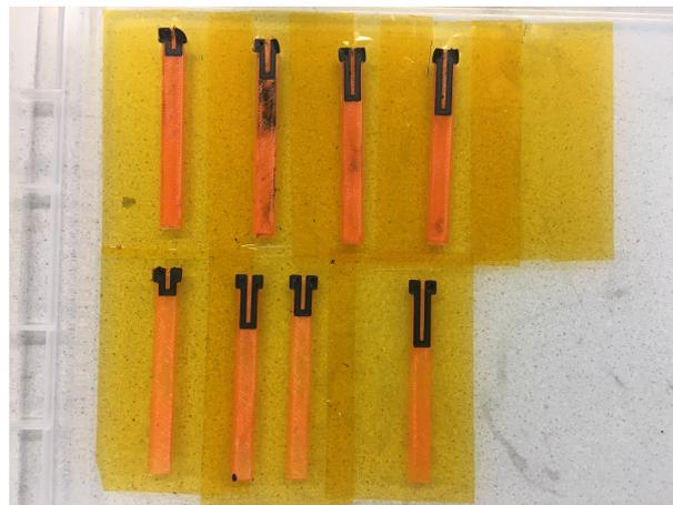
**Figure 3.3:** Printed sensors with strain gauge on the Kapton tape
