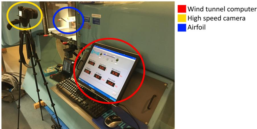
(b) Photo of the test set-up
