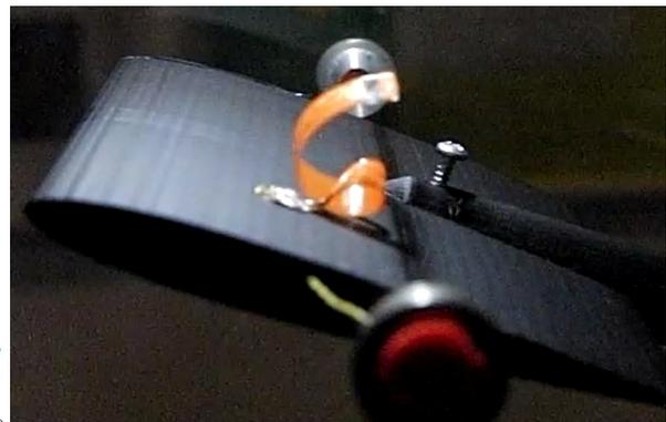
**(b)** Sensor with a gap and strain gauge length of 5 mm at AoA = 20°
