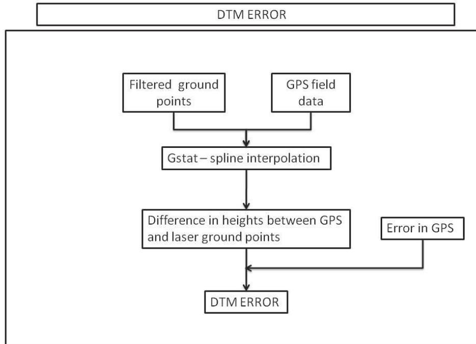
**Figure 3-8: Flowchart showing the process of finding DTM error**
