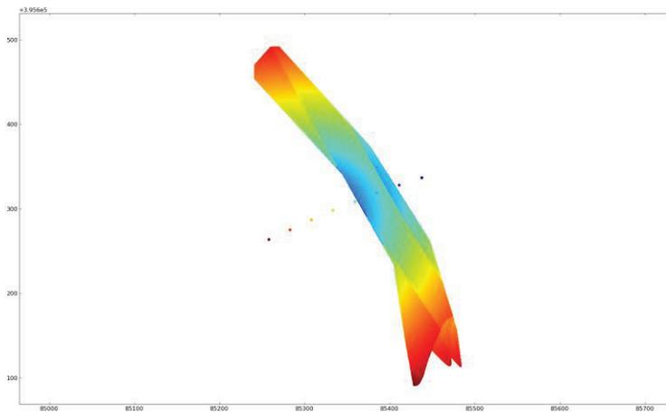
**Figure4-1: Flight path(dots) and laser echoes of a road showing variation in scan angle along with the flight path**
