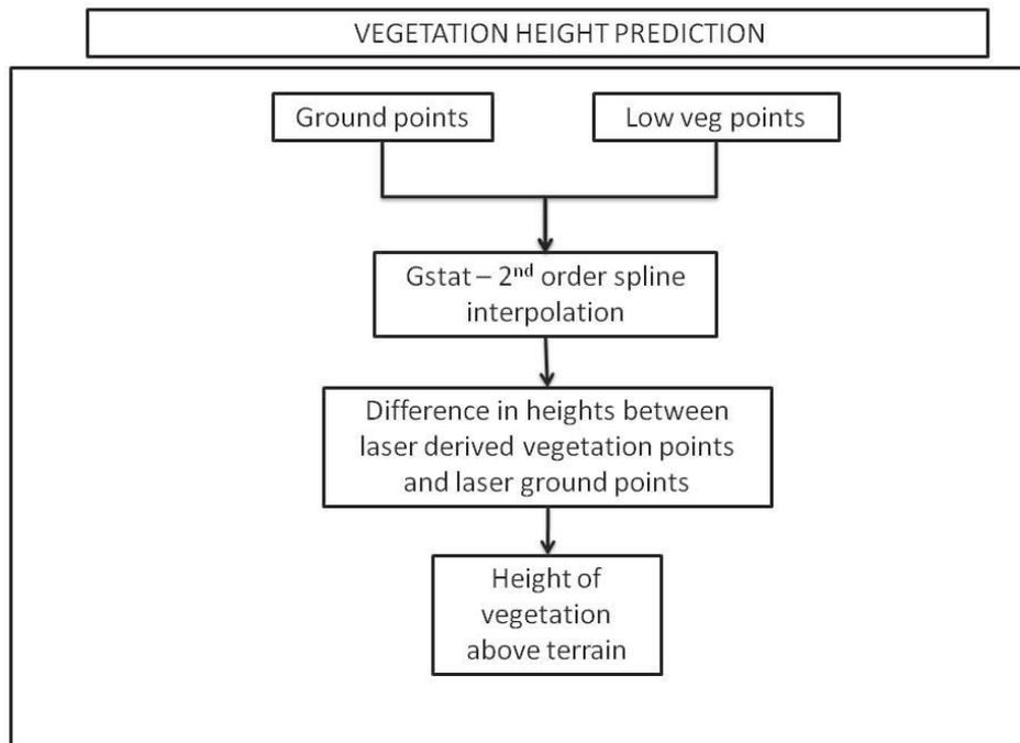
**Figure 3-9: Flowchart showing the process of finding vegetation height**
