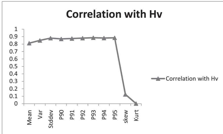
**Figure 5-1: graph showing strength of correlation between laser height data and various statistical measures**
