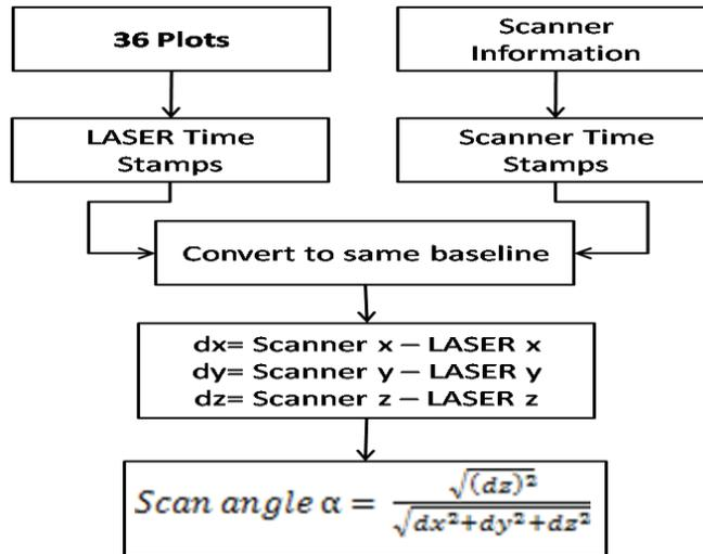
Figure 3-4: Scan angle workflow
