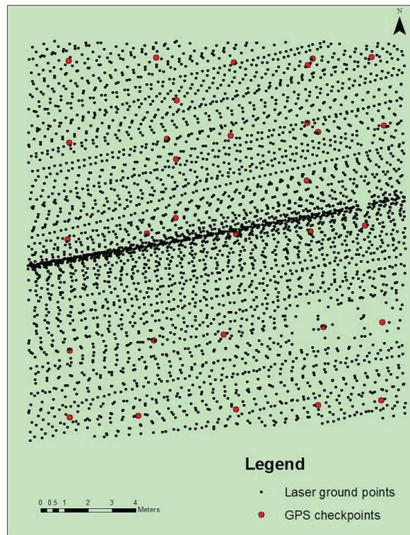
Figure3-7: dGPS checkpoints and laser derived ground points of the asphalt plot
