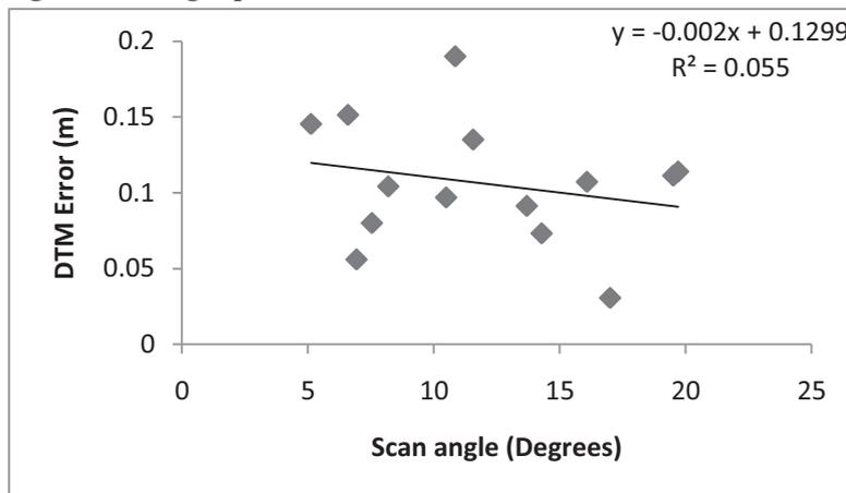
**Figure 4-2: Mean scan angle Vs mean DTM error**
