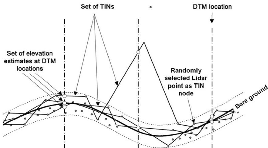
**Figure2-1 : repeated random selection of laser points used to build a set of TINs, out of which sets of elevation estimates are interpolated at the locations of DTM grid points. The remaining unfiltered vegetation points may become TIN nodes. (Kobler et al., 2007)**
