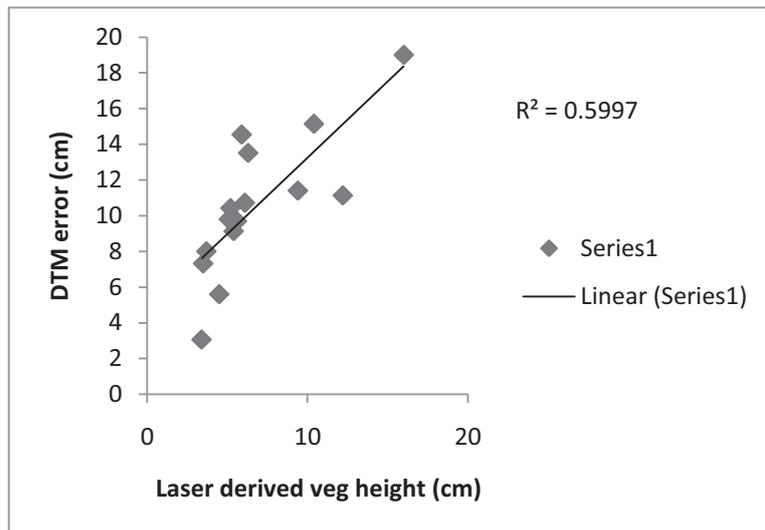
Figure 4-5: Plot between laser veg height and DTM error
