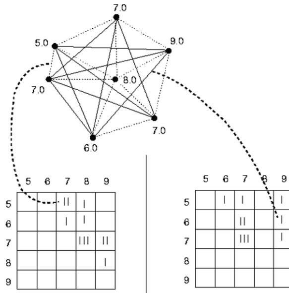
**Fig 2-2: GLCM on a point cloud texture Source: (Pfeifer et al., 2004)**
