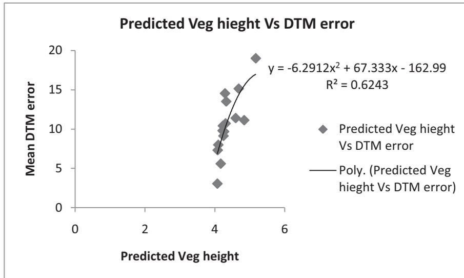
**Figure 4-6: Plot shown between predicted vegetation height using regression equation and DTM error**
