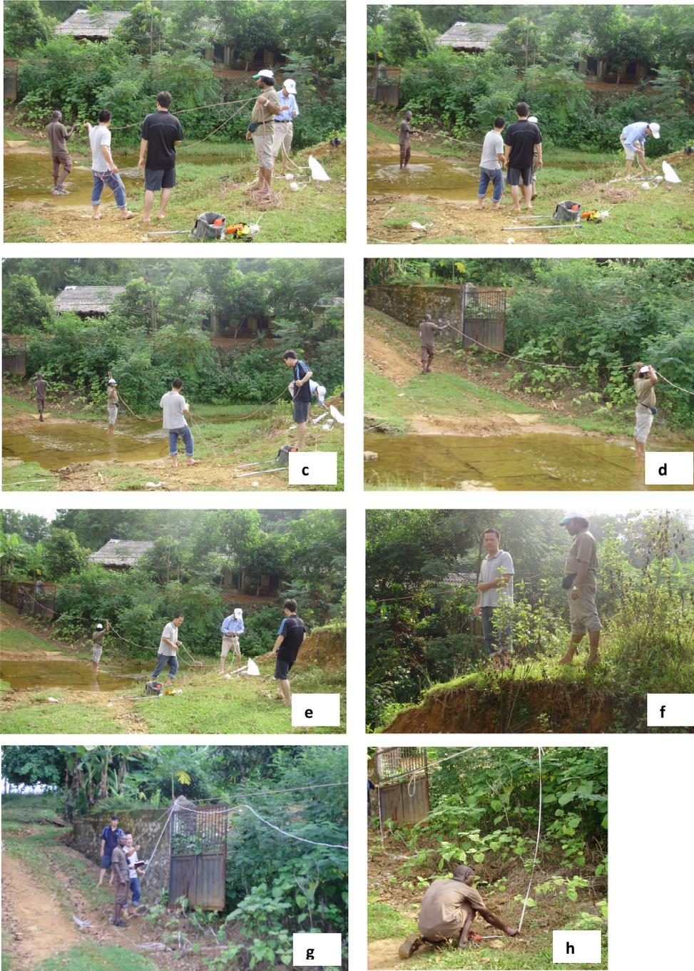
*Fig. 1 shows the stages in setting up and measuring of the spill-way cross section at the reservoir upstream of the catchment. The stages were; setting up the measuring lines (a-d), stretching the lines (e - f), and the actual depth measurement process (g - h).(source: fieldwork photographs September 2009).*
