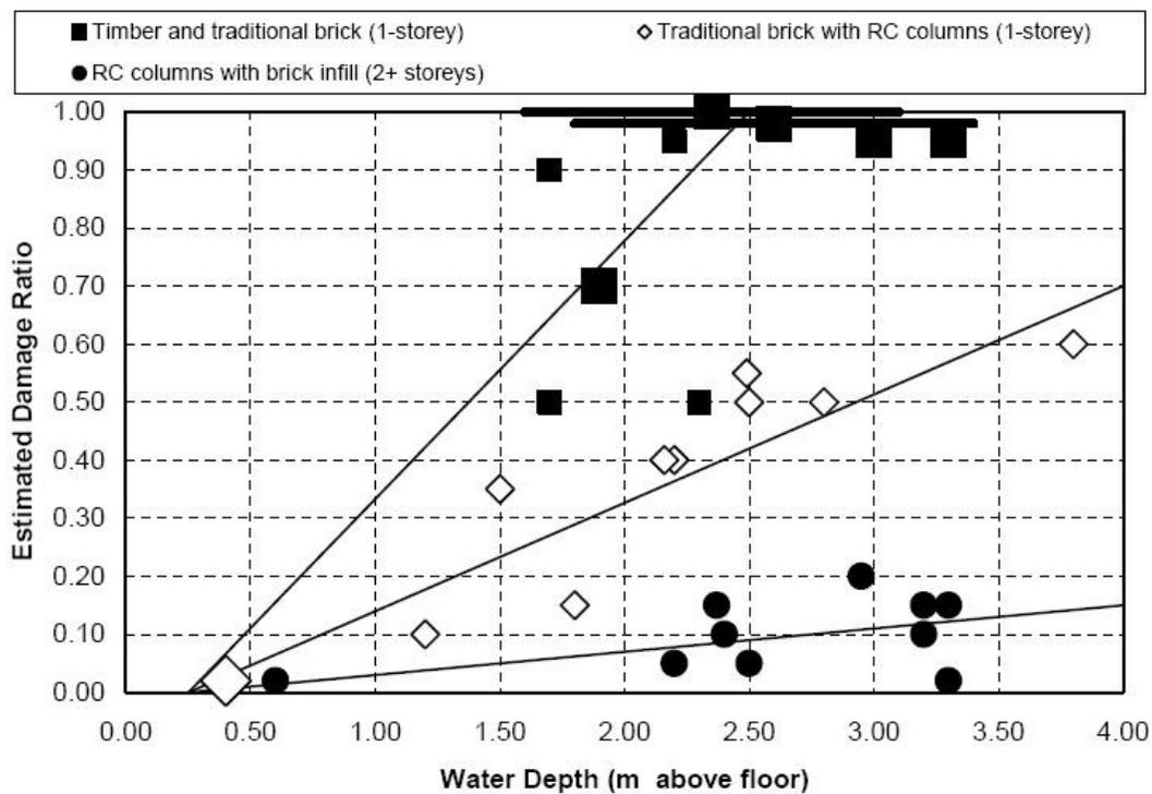
Figure 5-16. Estimated damage ratios and fragility curves as a function of inundation depth for various types of constructions (Reese *et al.*, 2007)
