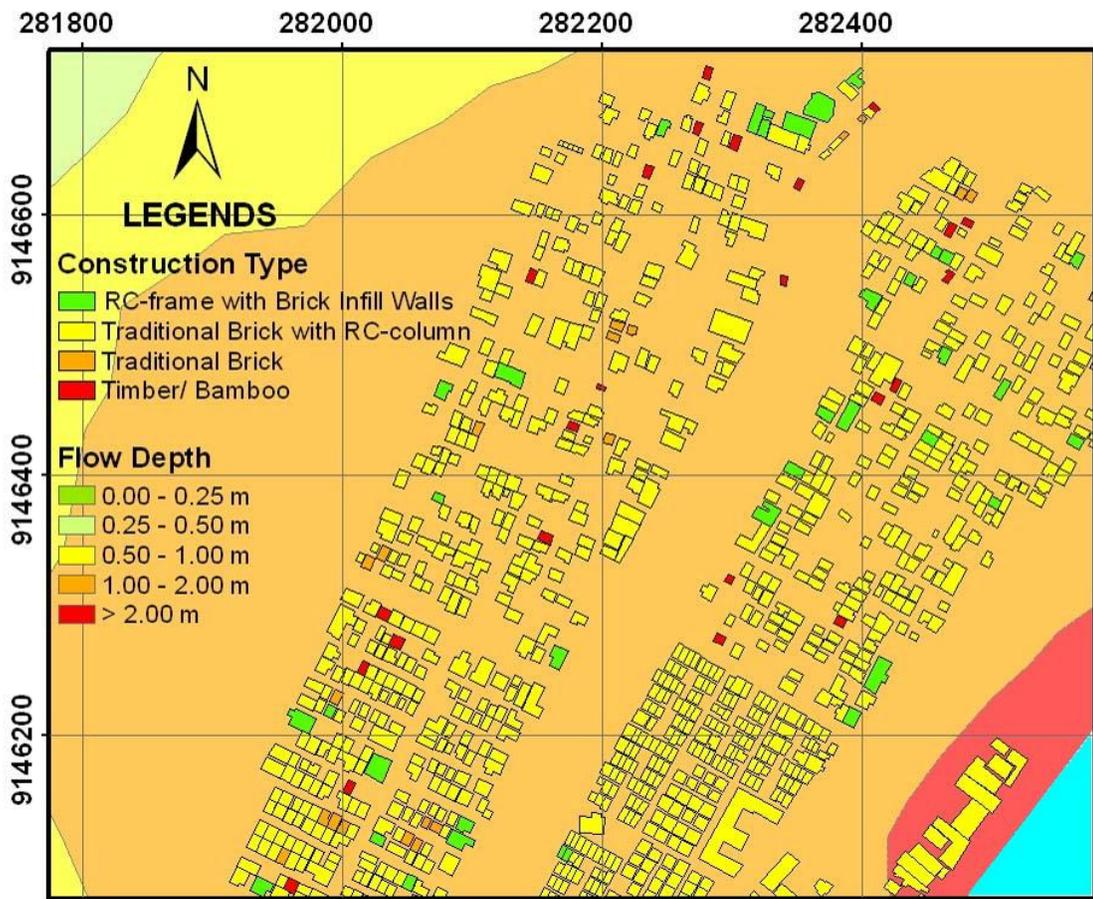
Figure 6-3. Various construction types located in various flow depth classes
