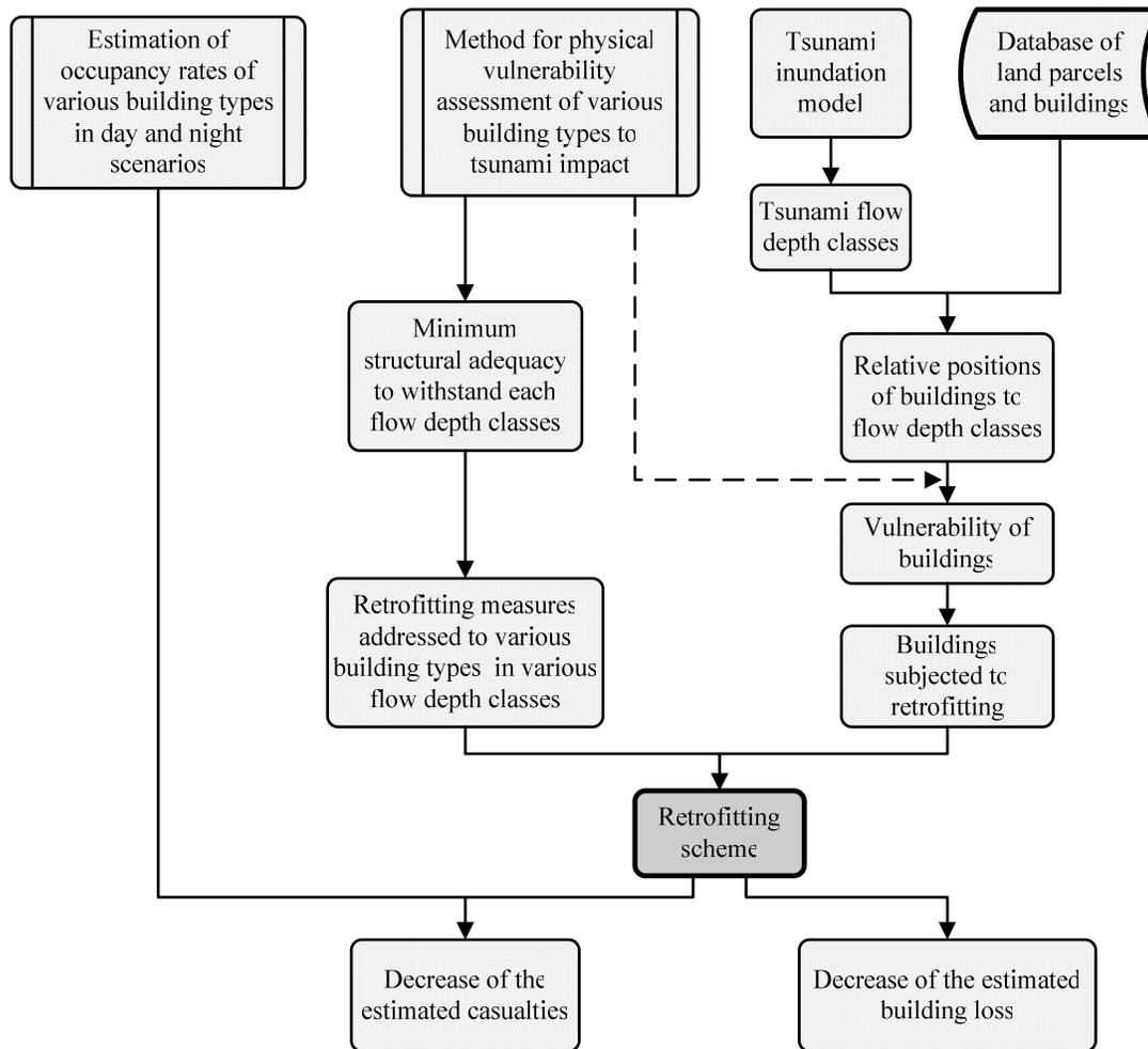
Figure 3-5. Structural mitigation planning: retrofitting
