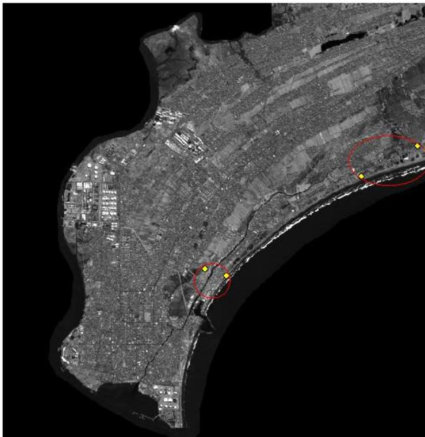
Four check points are chosen to compare the positional accuracy given by the two aforementioned geo-referencing methods. The comparison of the positional accuracy will show how significant those 17 extra GCPs on the sample areas contribute to improve the positional accuracy of the image. Two check points are located in the urban sample area and other two check points are located in the rural sample area, as shown in Figure 5.5.
