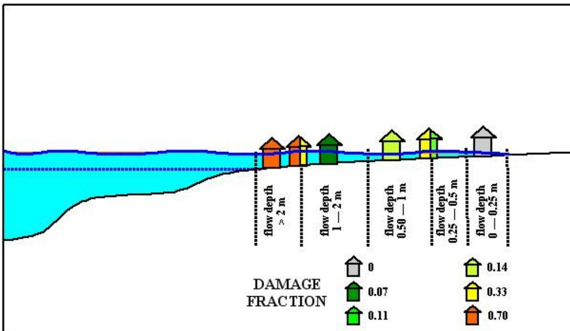
Figure 6-2. Illustration: various damage levels of buildings to tsunami flow depth
