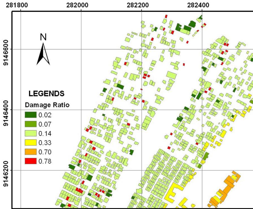
Figure 6-4. Various estimated damage levels of buildings
