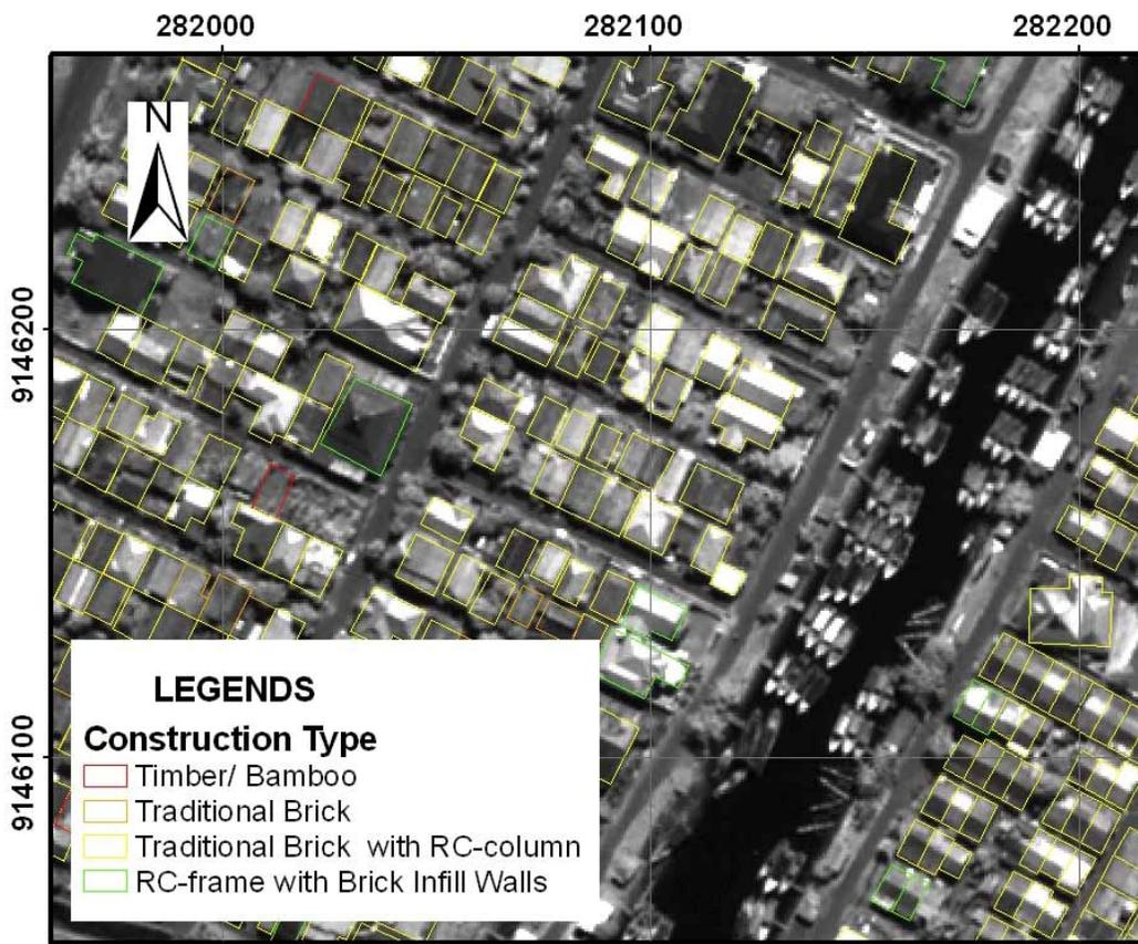
Figure 5-20. Various construction types in the newly generated individual building map overlaying the QuickBird imagery
