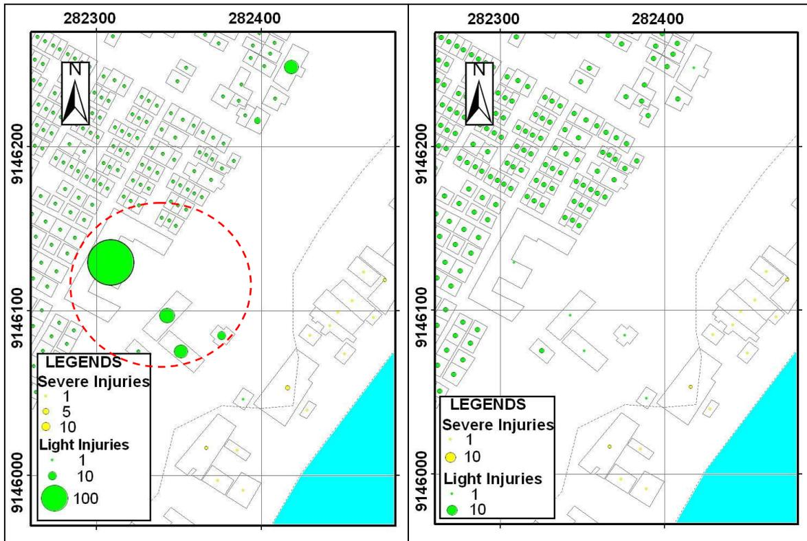
Figure 6-14. Estimated rates of severe injuries and light injuries in day time scenario after retrofitting (left), and estimated rates of severe injuries and light injuries in night time scenario after retrofitting (right)
