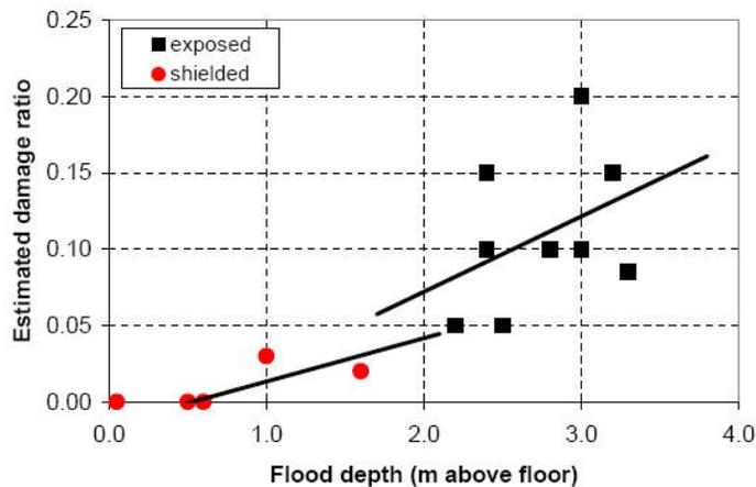
Figure 5-19. Damage ratios and fragility curves as a function of inundation depth and exposure for RC-frame with brick infill (Reese *et al.*, 2007)
