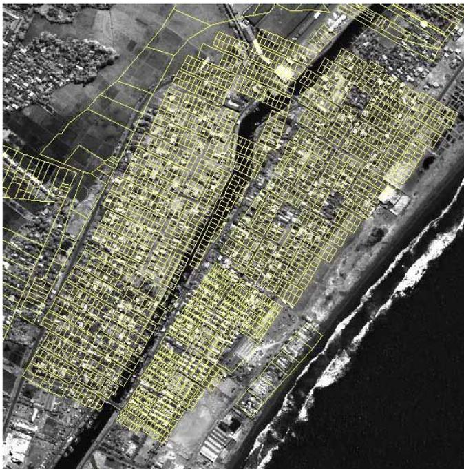
Figure 5-9. The Tax Office's block map overlaying the QuickBird imagery (2)
