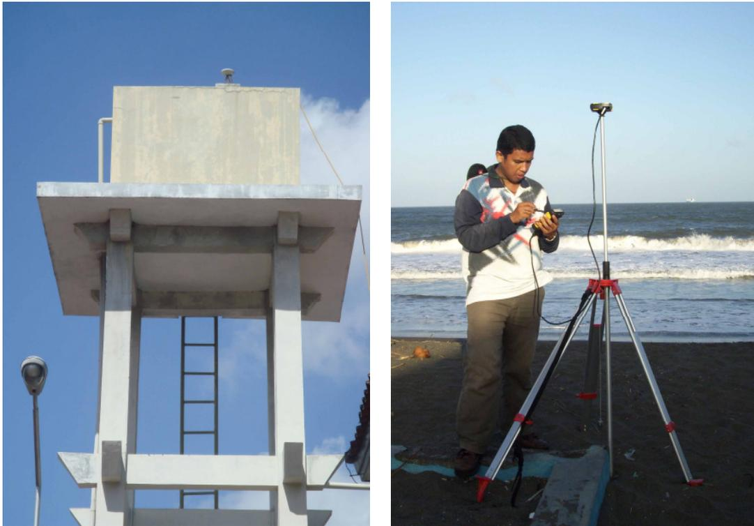
Figure 5-1. The base receiver at the reference station mounted on the top of a tower (left) and the GCP located on the edge of a structure identifiable on the imagery (right) (fieldwork doc.)
