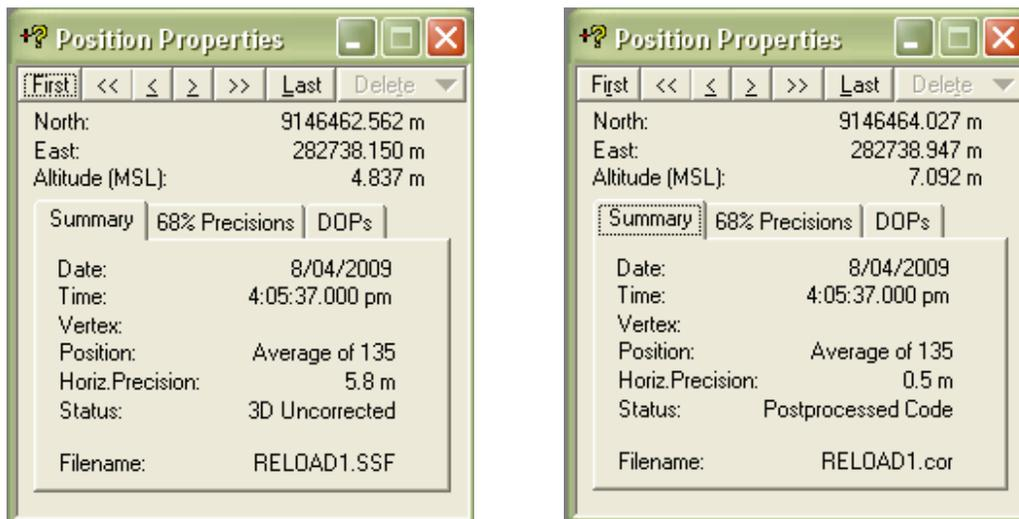
Figure 5-2. Horizontal precision of GCP before correction (left) and after correction (right)
