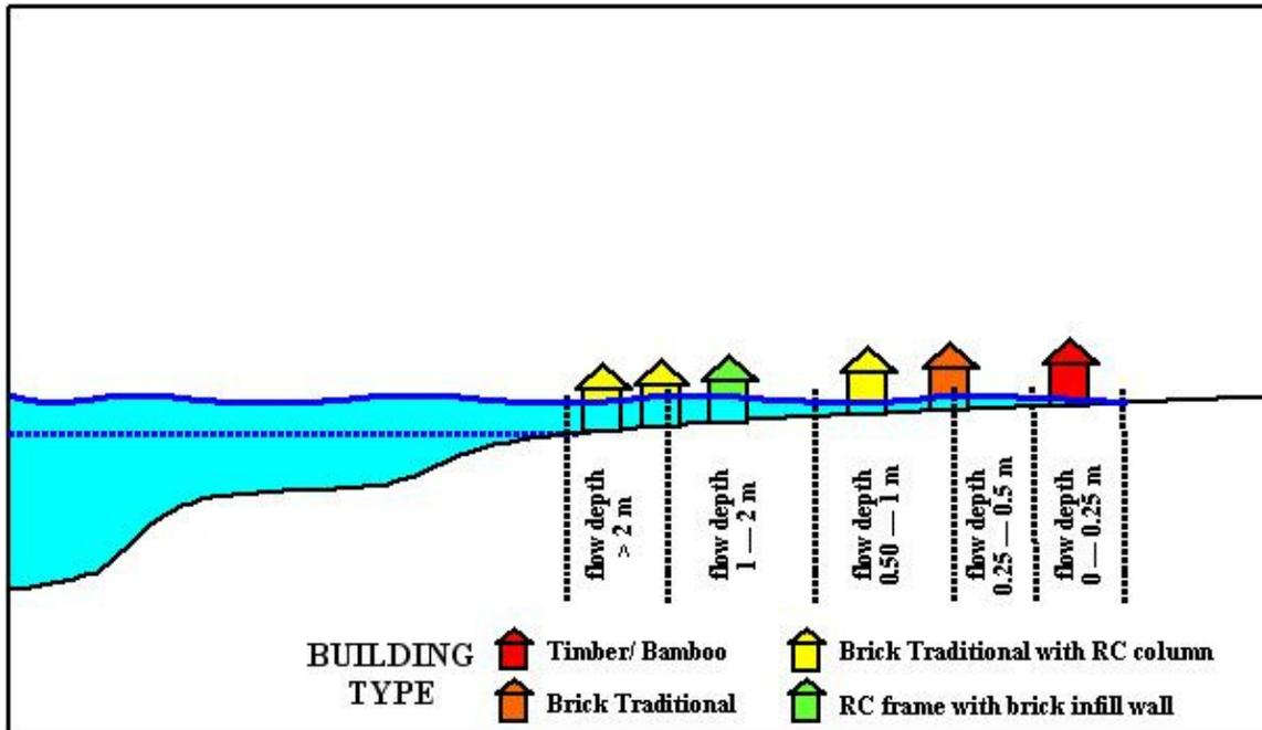
Figure 6-1. Illustration: various construction types inundated by various flow depth classes
