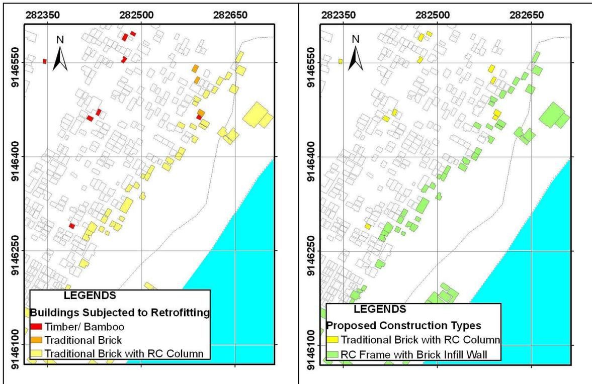
Figure 6-13. Buildings subjected to retrofitting because of the potential to contribute severe injuries and deaths (left), and the proposed changes on construction types to avoid death toll and severe injuries (right)
