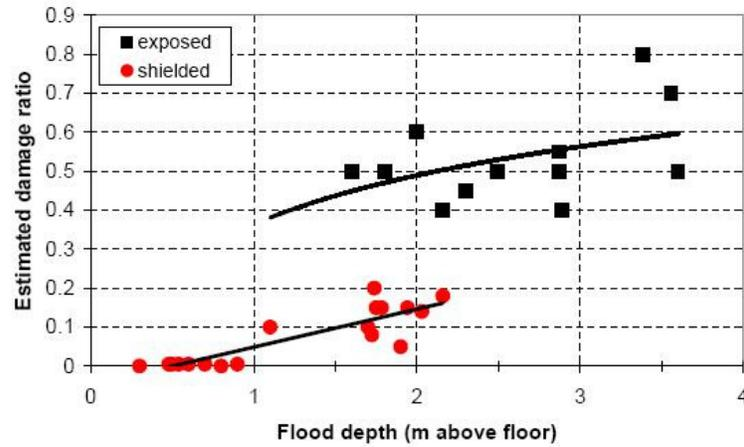
Figure 5-18. Damage ratios and fragility curves as a function of inundation depth and exposure for traditional brick buildings with RC-columns (Reese *et al.*, 2007)
