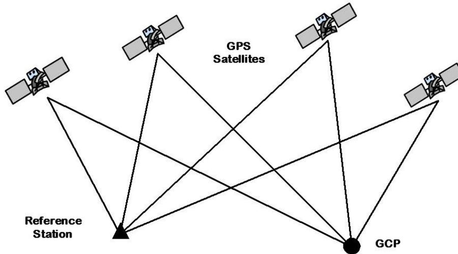
Figure 2-2. Illustration of Differential GPS measurement
