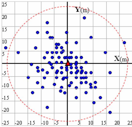
Figure 2-1. Illustration of positional accuracy specified by CE90
