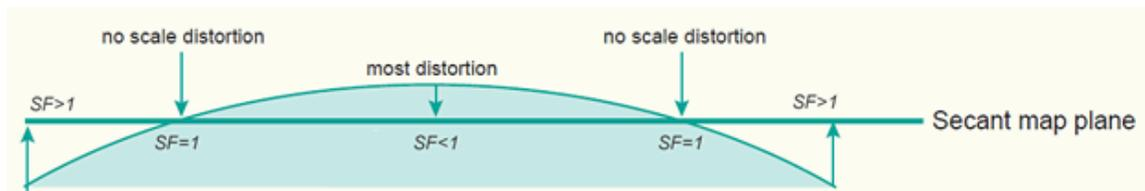
Figure 5-6. Scale factor on a secant map plane (Knippers, 1999)
