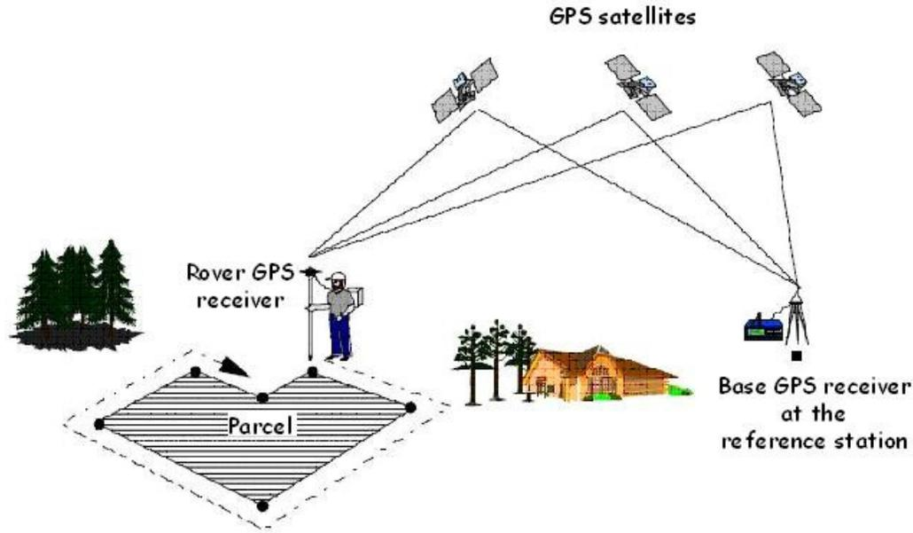
Figure 6-20. Real Time Kinematic GPS technique for parcel reconstruction (Abidin, 2007)
