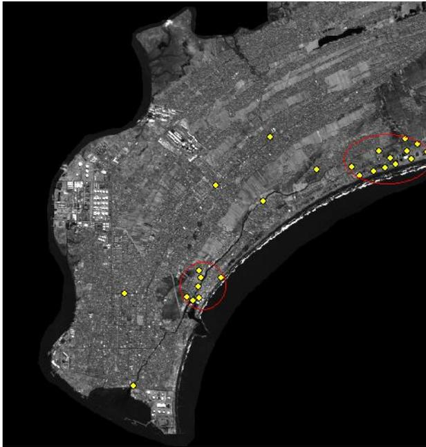
Eight GCPs which are spread over the study area and 17 extra GCPs located in the two sample areas are used for the second geo-referencing method. Extra GCPs are expected to reduce the positional error to the minimum. The spreading of the GPS is shown in Figure 5.4 on the left.
