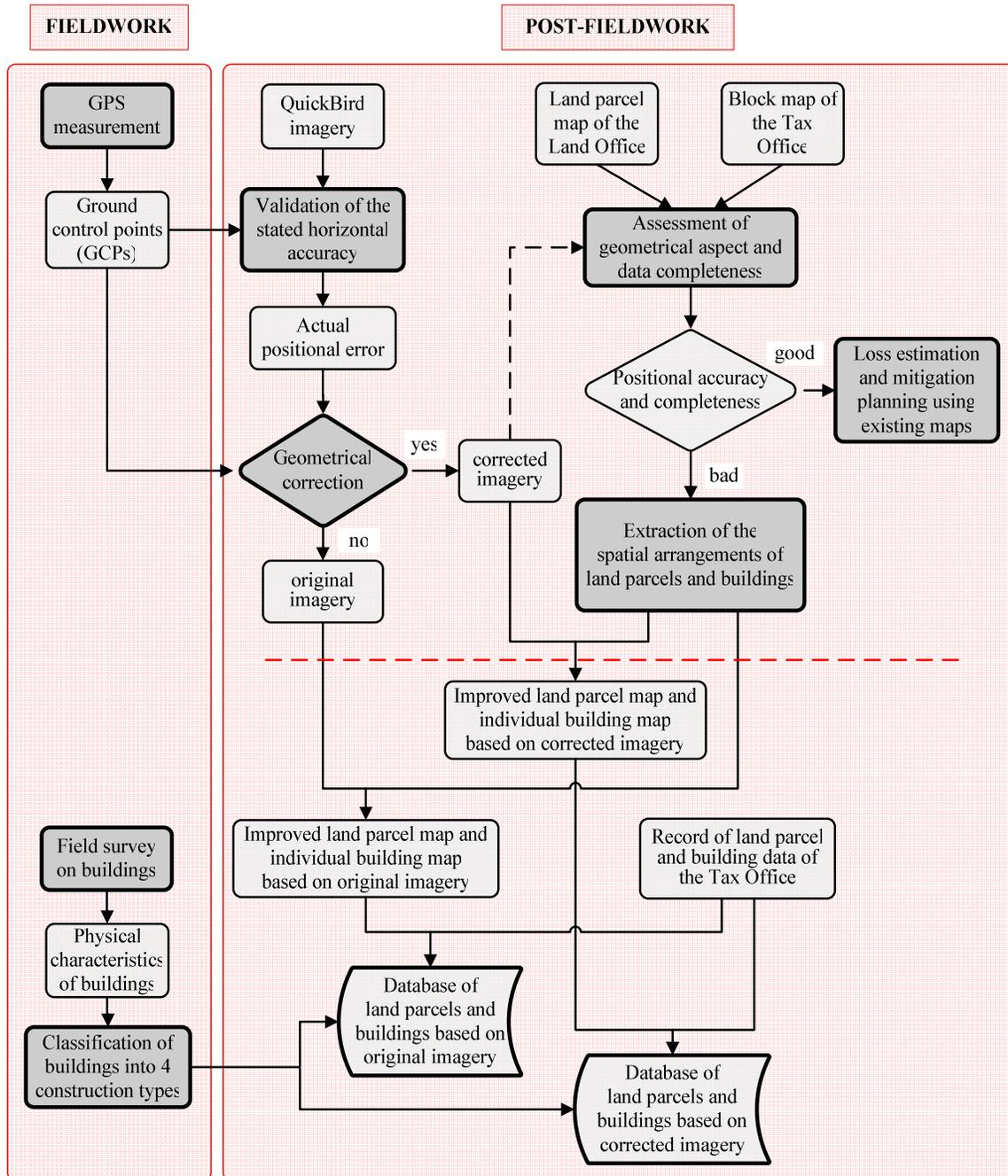
Figure 3-2. Generating the database of elements at risk
