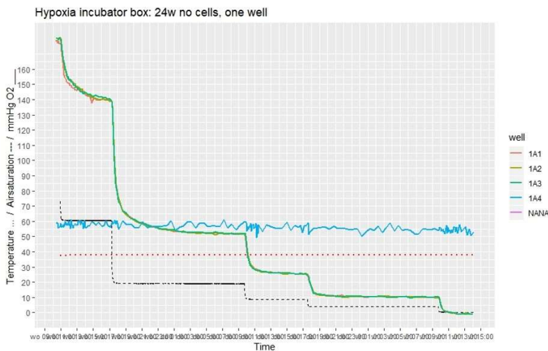
(b) Clear difference in received signal and determined PO 2 level when adjusting applied oxygen level of 8%, 5% or 0% oxygen within cell measurements from in house experiments.
