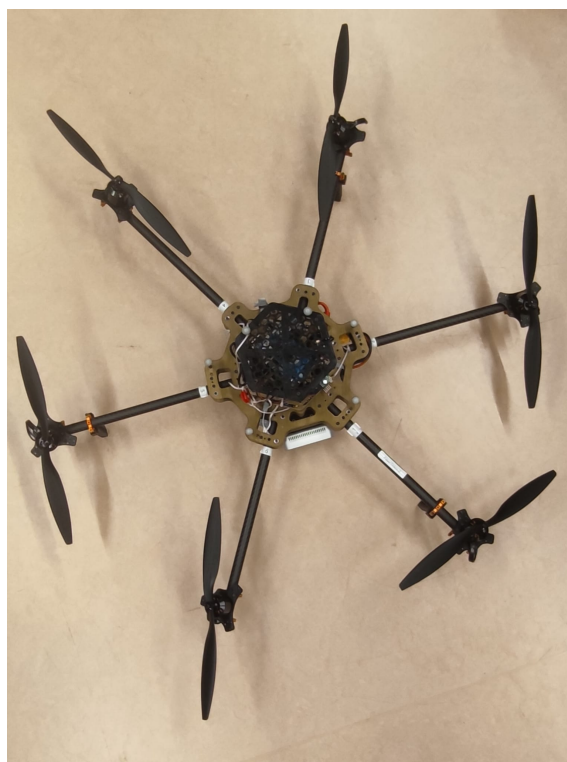
Figure 4.1: FiberTHex drone with 6 propellers and the camera D435i mounted between propeller 6 and 1.
