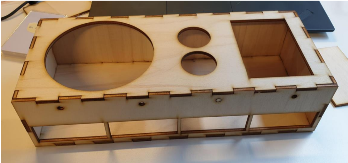
Figure 30 Lasercut plywood case put together
