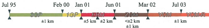
Figure 2: Configuration of the ERS-2 piloting modes and corresponding orbit dead-band evolution (Miranda et al., 2004)
