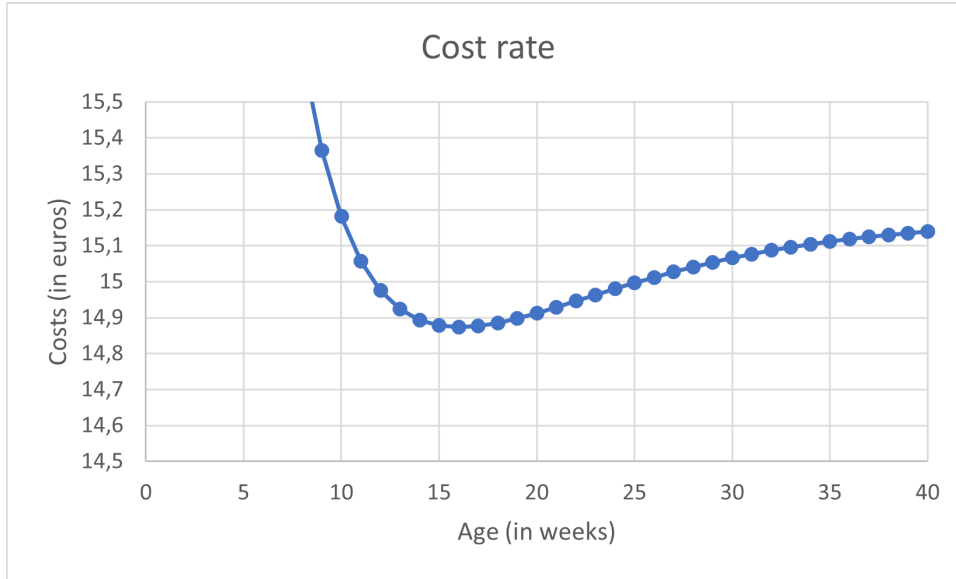
Figure 5.2: Optimal replacement age calculation for the Fans of Company X, Large locations
