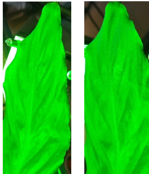
Figure 12A and 12B: Approx. twenty-four-hour leaf clamp test. No new visible defects could be found on the leaf.
