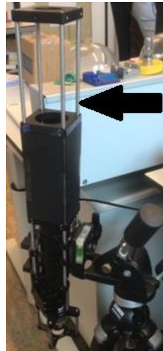
Figure 4: Image of the current microscope setup, provided by van den Berg. The black arrow points at one of the metal rods used for mounting. The leaf clamp will be mounted on the underside.
