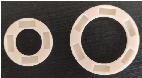
Figure 13: An overview of the bottom of both the small and large ring. The holes for the magnets have been adjusted to fit the larger ones.
