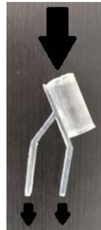
Figure 18: PAM mount: Printed in clear resin. PAM device goes into top where arrow points. Bottom legs go into the backplate and are screwed tight.
